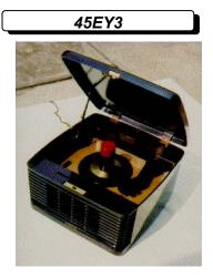
The bakelite case has pleasing lines and rounded corners which makes it a desirable piece of 1950's memorabilia today. Inside it has a 3 tube amplifier and 4X6 inch speaker. This gives it a decent amount of volume, but the sound is definitely on the tinny side.
