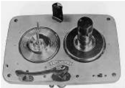
FIG.2 One tonearm uses either of two turntables
