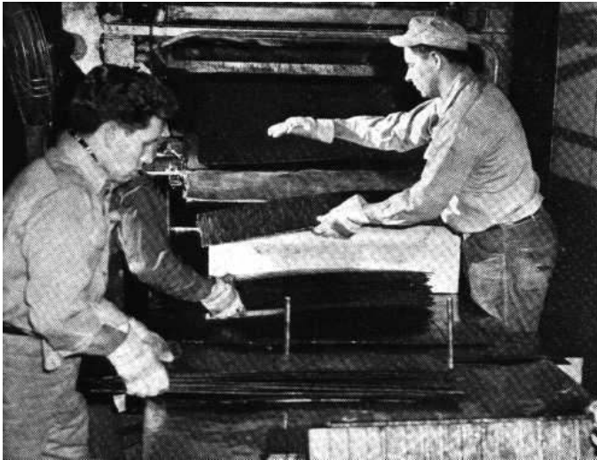
1) Sheets of translucent plastic are reduced to proper thickness
