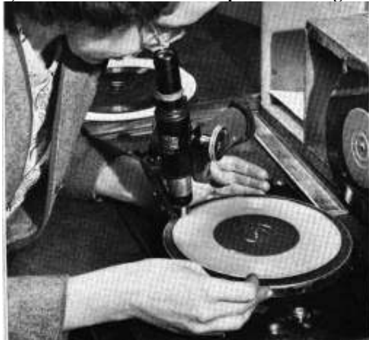
5) Exact centering of record is assured by checking the movement of the outer rim under a microscope.
