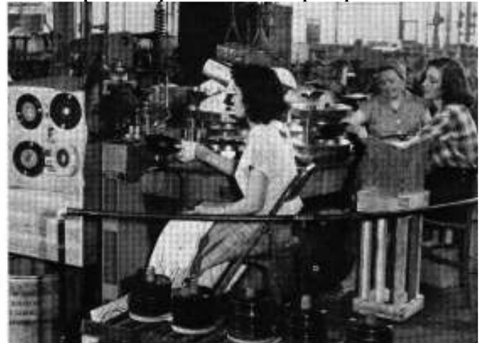
2) 45 rpm record complete with labels is removed from one of the powerful presses at Indianapolis plant
