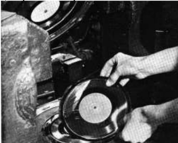
3) Excess plastic material called 'flash' is stripped from the outer rim.
