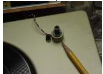
Where pencil is pointing, add extra washer under c-clip
