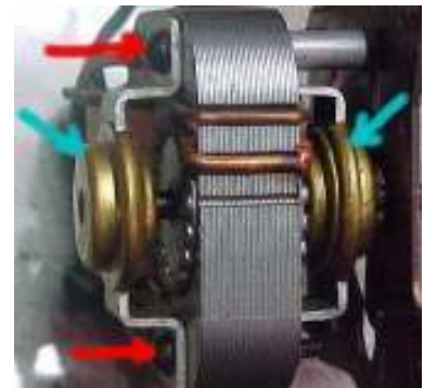
Blue arrow- bearing cups. Red arrow- mounting screws.
