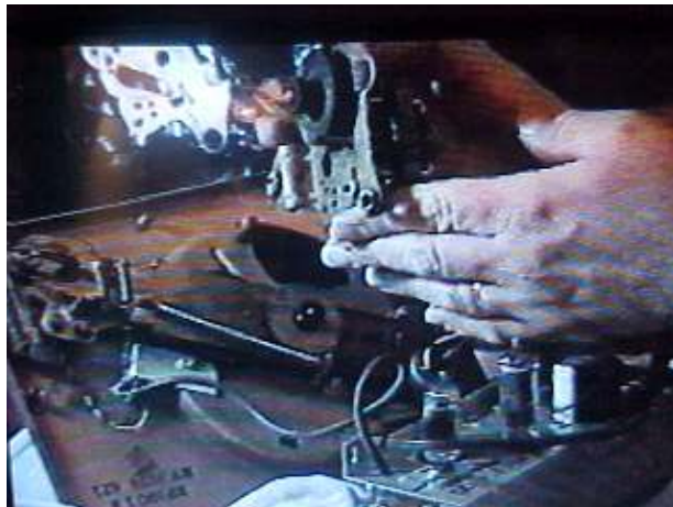
Removing motor on rp-190 changer
