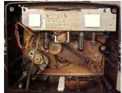
3 white reinforcements are glued in place
