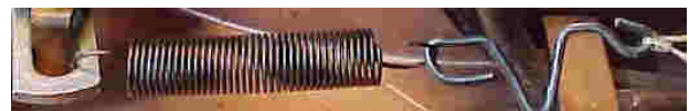
Changer slide switch in ON position, tension applied to idler holding it against the motor shaft.
