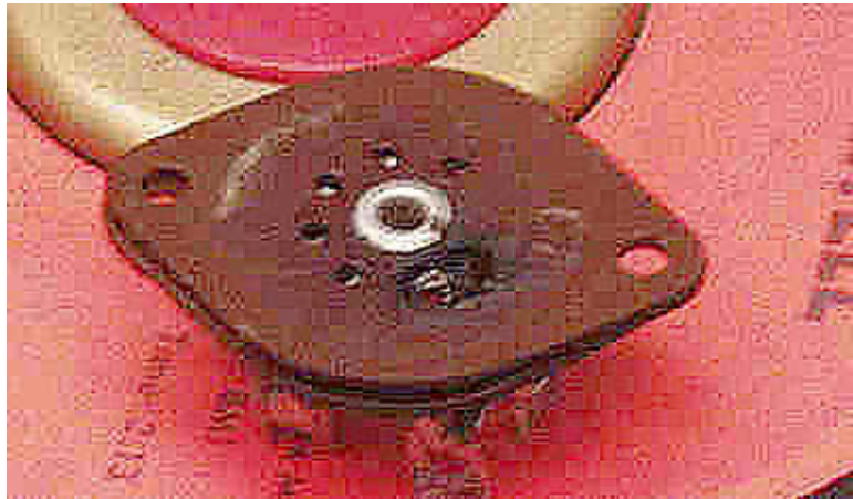
Internal Short between pins 1 and 2 created unexpected fireworks
