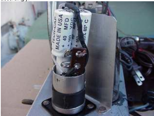
Picture 2 showing replacement capacitors stuffed tightly. The existing terminal connectors could not be used because not only they were aluminum, but for some reason there was a
