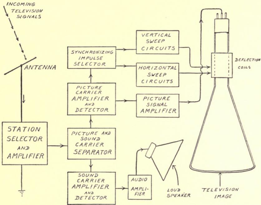
FIG. 53—Plan of a television receiver.
