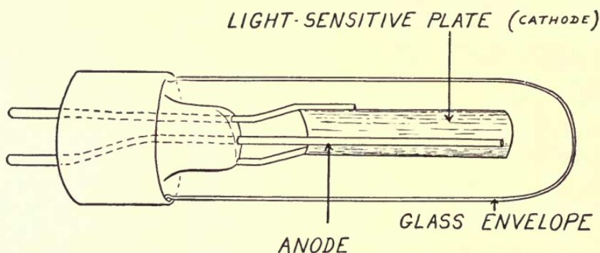
FIG. 3—Construction of a photoelectric cell.
