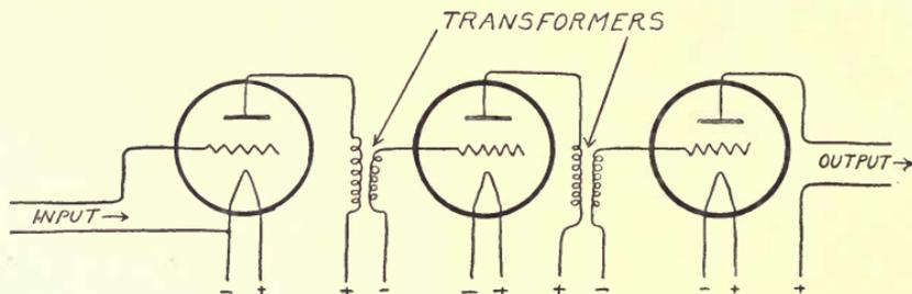
FIG. 22—Use of a series of three vacuum tubes (represented by circles) with transformers in a circuit to amplify television signals.
