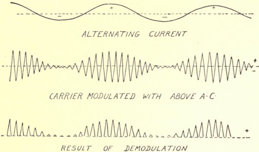
FIG. 24—Amplitude modulation of a carrier current.
