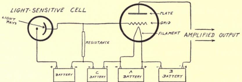
FIG. 20—A vacuum tube (represented by the larger circle) used as an amplifier of the light modulated current produced in a light-sensitive cell (represented by the smaller circle).
