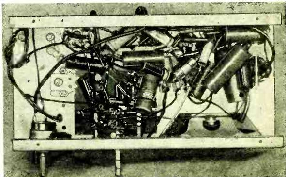
During these adjustments the loop should be placed in the *exact position* with respect to the chassis that it will occupy when the set and loop are mounted in the cabinet.
