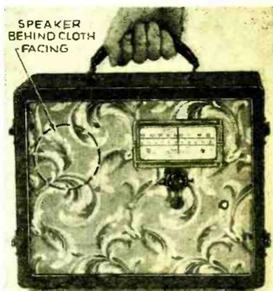
Panel of 4-tube broadcast band portable.
