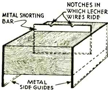
Fig. 7—Sliding block used to short Lecher wires.
