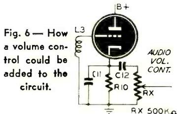
Fig. 6—How a volume control could be added to the circuit.
