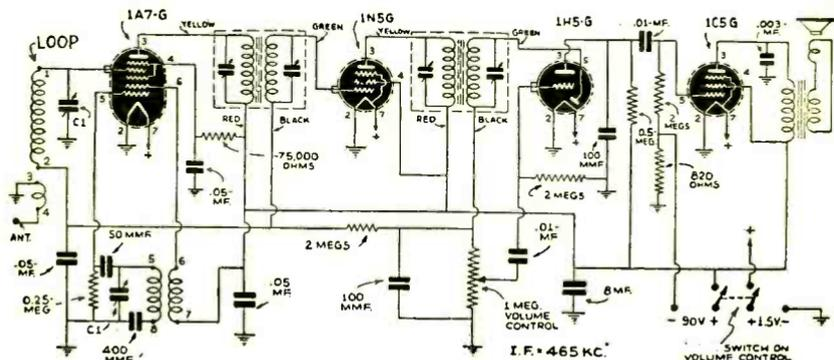
Fig. 1—Set wired for battery operation.
