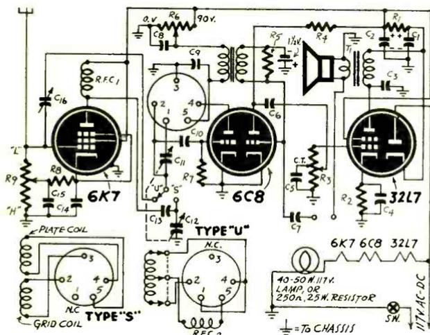
Fig. 1 — Schematic shows switching and plug-in combined.
