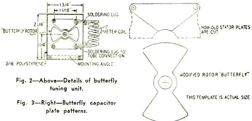
Fig. 2—Above—Details of butterfly tuning unit.
