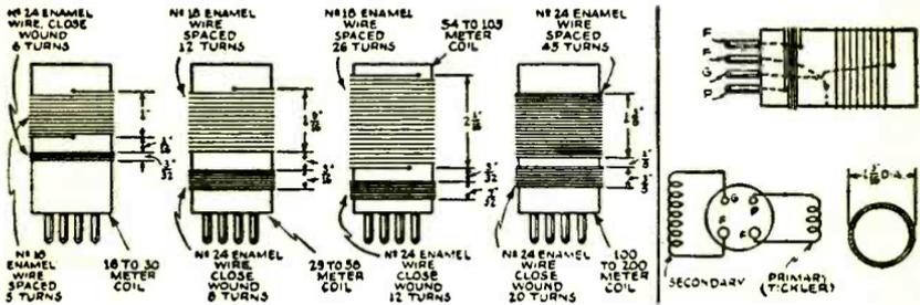
Fig. 1—Coil winding data for Twinplex.
