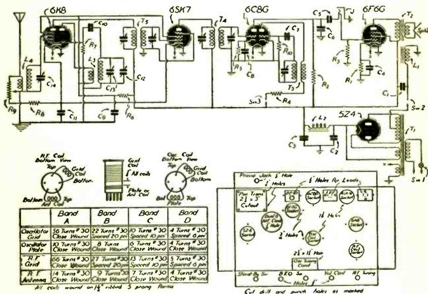
Fig. 1—Short-wave coil data is given at left of diagram above.
