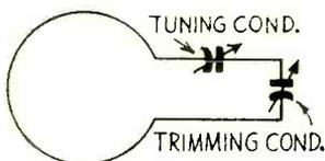
Fig. 5—Absorption wavemeter circuit.
