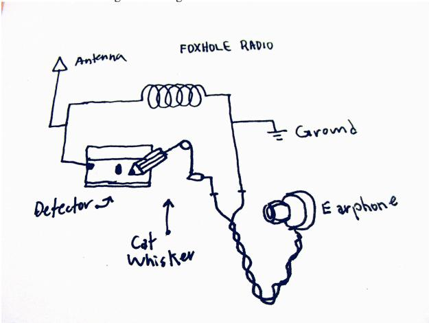
Hook it all together – I used brass tacks to keep it all together and paperclips to connect all the wires.
