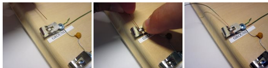
Figure 16. To connect a wire to a Fahnestock clip, first press down on the tab of the clip with your finger. Use your other hand to thread the end of the wire through the clip, as pictured, then release the tab.
