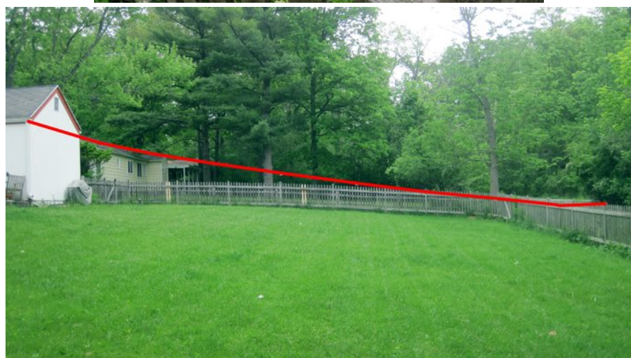
Figure 14. An antenna strung up between the gutter of a house and a wooden fence in a back yard (the antenna is highlighted with a red line in the bottom photo, since the wire is too thin to see easily). This antenna is about 60 ft. long.
