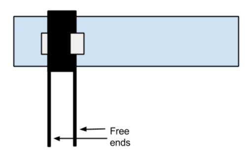
Now use 15m of wire to build another coil right next to the first one, but this second coil needs to be **fifty turns** long. Be careful; it is very easy to get the wire tangled and you don't want any knots in it. Again, make sure that the turns are all tight up against one another, and use tape to hold the first and last turns in place. When you are finished it should like like this:
