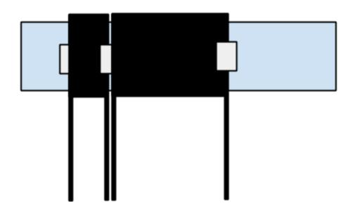
Cut the four tails so that they are each about 10-15cm long, and use wire strippers to remove ~1cm of insulation from the end of each one.
