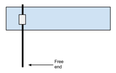
Then wind the wire around the tube **ten times** making sure that each turn is tight up against the previous turn. There should not be a gap between the wires on each turn and they should not be slack on the tube or crossed over other wires. After ten turns, secure the last turn with another piece tape and leave another tail of about 20cm.
