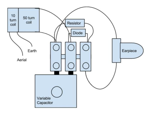
Your earpiece may have a 3.5mm plug on the end of its cable. If it does, cut it off and use wire-strippers to bare 1cm of the ends of the two wires just as you did with the coil tails.
