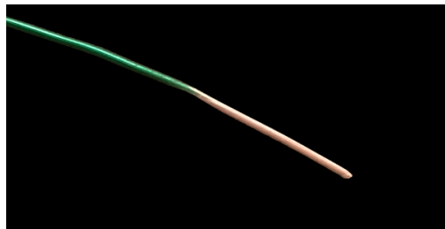
Figure 6: Sanded Wire End
