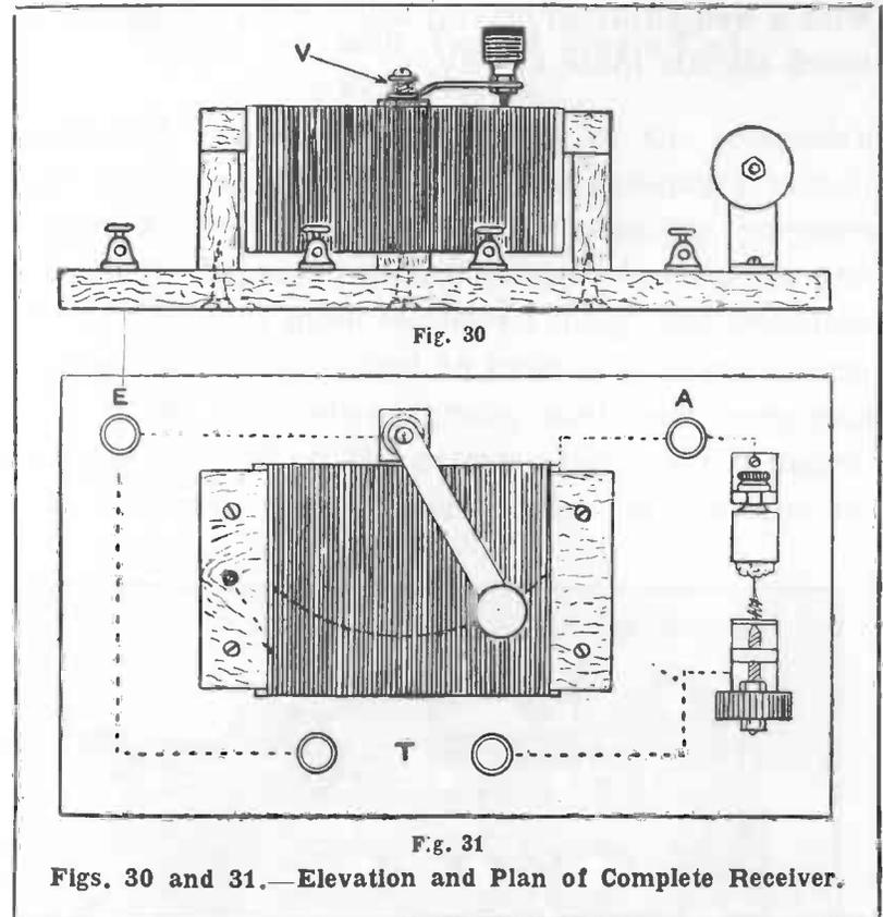
Figs. 30 and 31.—Elevation and Plan of Complete Receiver.
