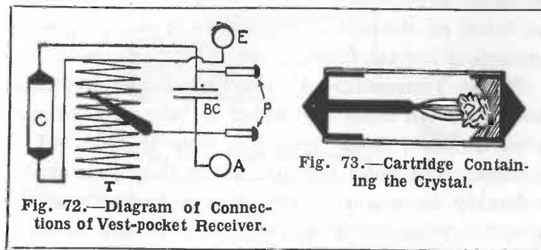
**The Tuning Coil.**—To the under side of the ebonite panel is fitted the tuning inductance, which consists of No. 32 enamelled wire wound on an ebonite former  $\frac{3}{16}$  in. thick, 2 in. deep, and as wide as can be got into the case, that is, a shade smaller than the ebonite panel itself.
