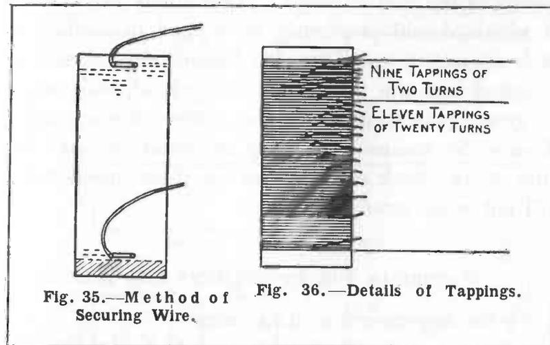
Fig. 35.—Method of Securing Wire.
