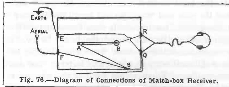
Fig. 76.—Diagram of Connections of Match-box Receiver.
