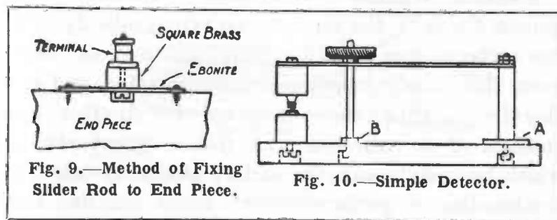
being cut away to accommodate the head of the terminal screw. The screw is put through the ebonite, passed through the hole in the square brass, and the two parts of the terminal are screwed up tightly. The same process is repeated at the other end of the square brass, and the pieces of ebonite are then screwed to the ends.
