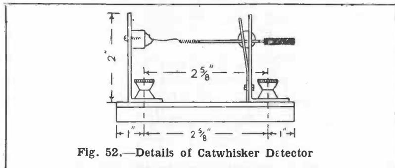
Fig. 52.—Details of Catwhisker Detector
