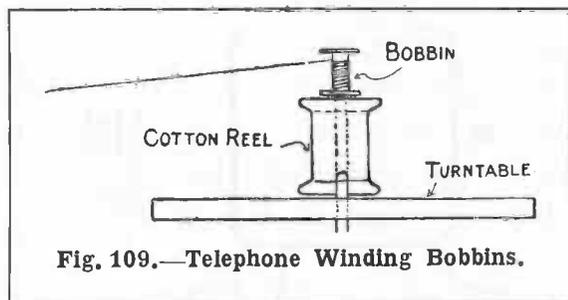
is to be wound and fix it to the top of the reel by means of a spot of glue or sealing-wax. The wire can then be attached to the bobbin and the turntable allowed to revolve as in Fig. 109. The speed at which it revolves can, of course, be regulated by the controller which is fitted to most gramophones.
