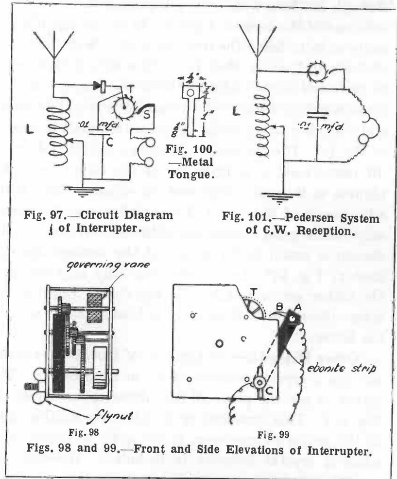
$c$  to accommodate the bolt. The tongue  $B$  is cut to the shape shown in Fig. 100 out of springy sheet brass about the thickness of drawing-paper. An ordinary pair of scissors will cut the brass quite easily, and the
