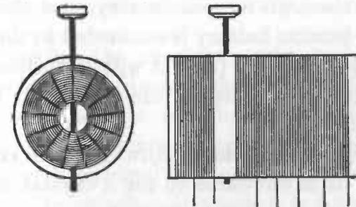
Fig. 64.—End and Side Views of Mounted Reaction Coil Fitted in Inductance Coil.
