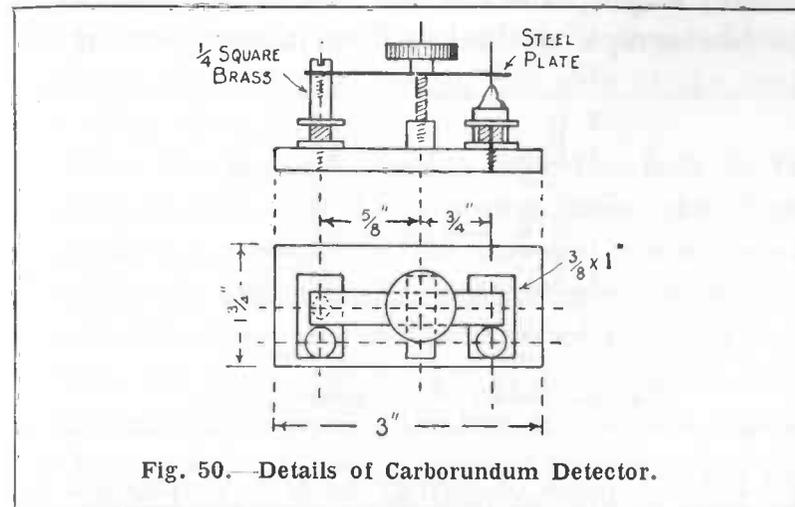
Fig. 50.—Details of Carborundum Detector.
