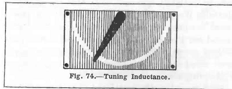
**The Contact Finger.**—A small contact finger is now made up, soldered to a short spindle, and arranged to make contact on the bared portion of the inductance
