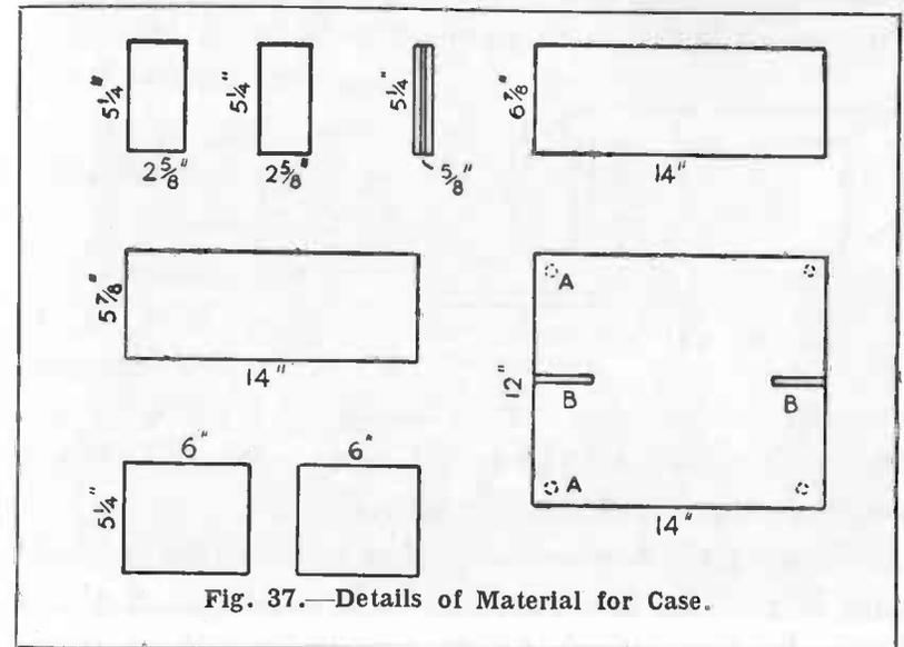
Fig. 37.—Details of Material for Case.
