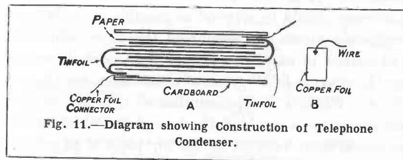
Fig. 11.—Diagram showing Construction of Telephone Condenser.
