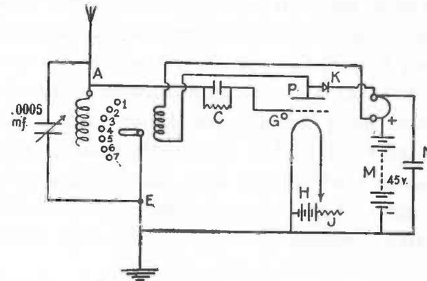
Fig. 65.—Diagram of Connections for Complete Receiver.
