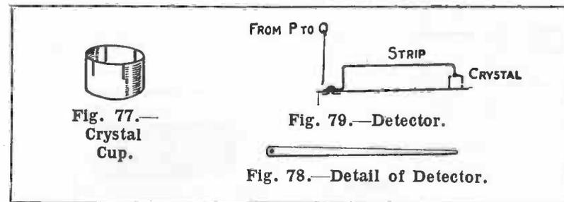
shown in Fig. 79, and fasten it with a fastener at the proper distance from the cup.
