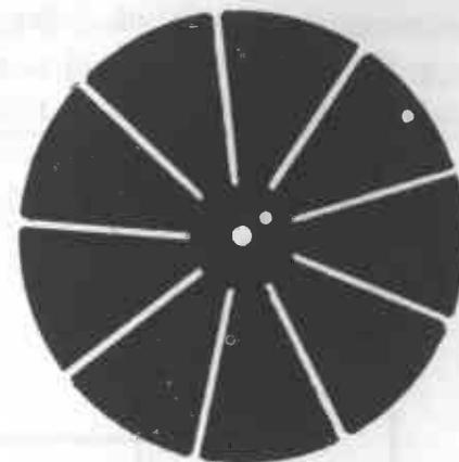
Fig. 60.—Tuning-coil Former.
