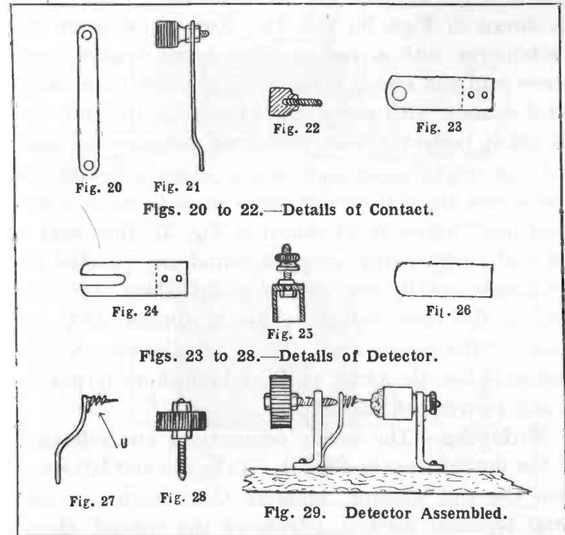
rounded off to a point. The general arrangement of the detector is clearly shown in Fig. 29.
