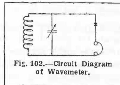
Fig. 102.—Circuit Diagram of Wavemeter.
