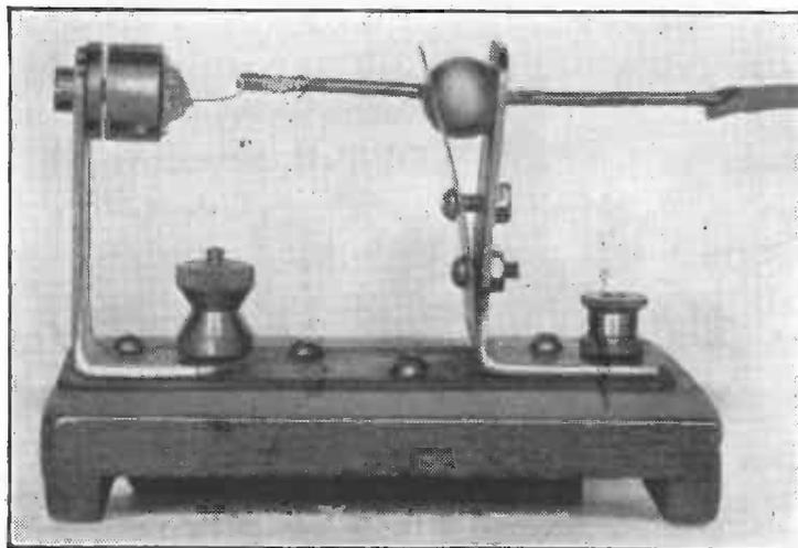
Fig. 53.—Photograph of Catwhisker Detector.
