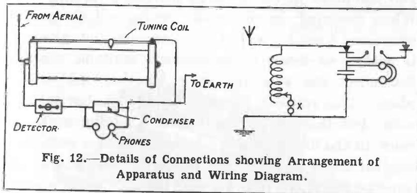
Fig. 12.—Details of Connections showing Arrangement of Apparatus and Wiring Diagram.
