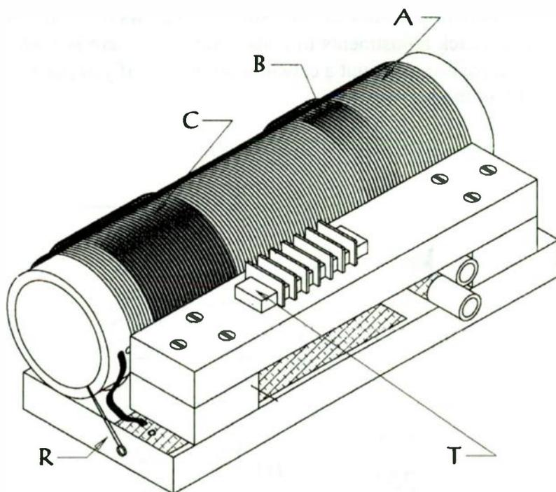
Figure 5: Pictorial view, *A*-tuning coil, 126 turns of 18 gauge plastic coated wire; *B*-10 turns 18 gauge wire over tuning coil; *C*-25 turns 18 gauge wire over tuning coil; *T*- terminal block; *R*-rubber band.
