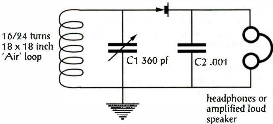
Figure 1: Schematic
