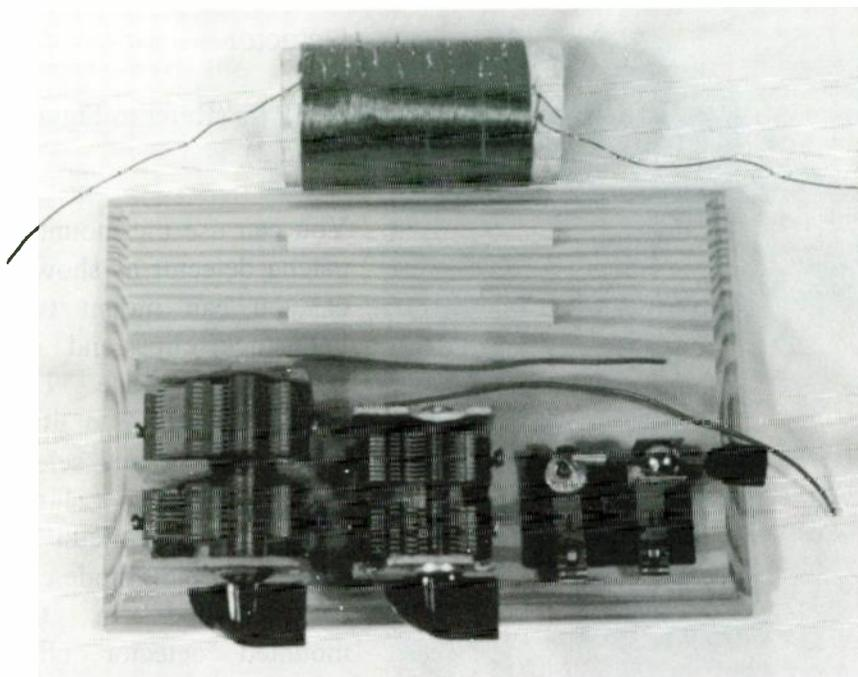
Photo 3: Location of coil mounting strips
