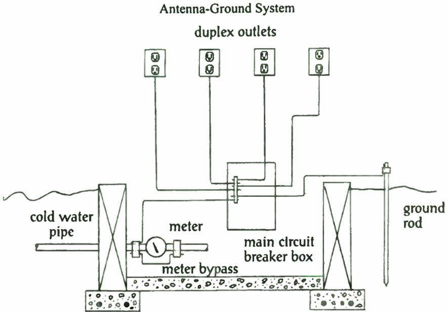
Figure 4: Typical residential equipment grounding scheme
