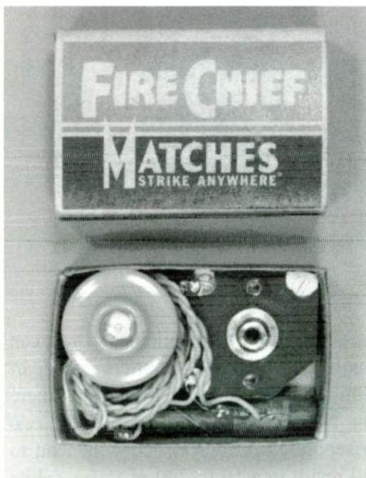
Photo 2: Matchbox crystal radio in box
