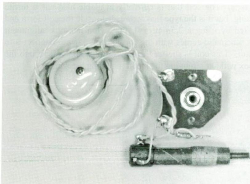
Photo 1: Matchbox radio parts
