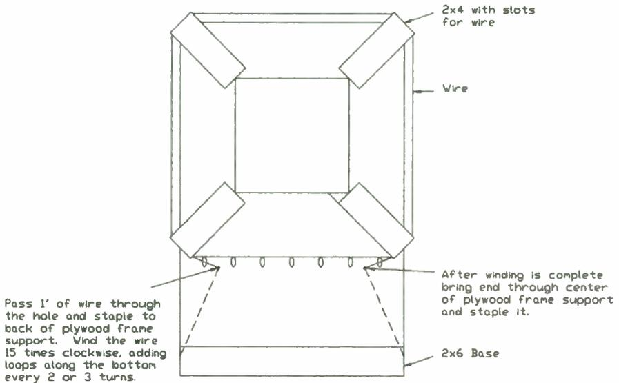
Figure 4: View of wire added to frame
