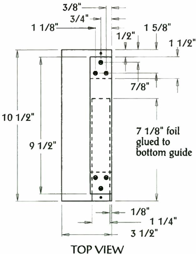
Figure 4: Guide measurements
