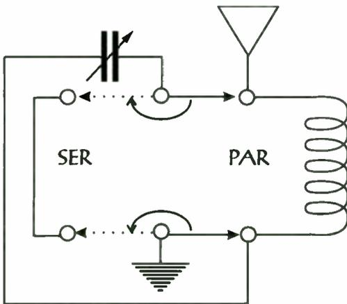
Figure 6: Switching between parallel resonant and series resonant circuit
