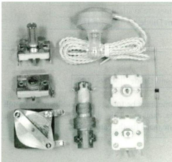
Photo 3: Top and center left, two trimmer capacitors; top center, crystal earphone; bottom left, variable capacitor; bottom center, coil; bottom right, two enclosed variable capacitors; far right, diode.
