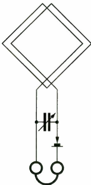
Figure 1: Schematic of the krystal kludge set
