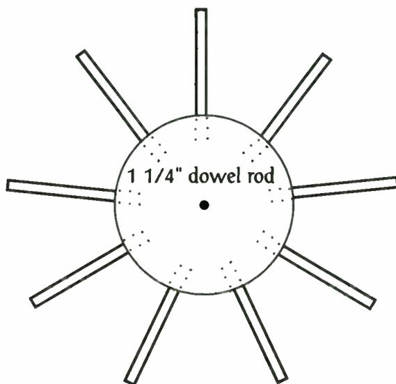
Figure 2: Coil form, 9 dowel rods,  $\frac{1}{4}$ " diameter, approximately 6" long
