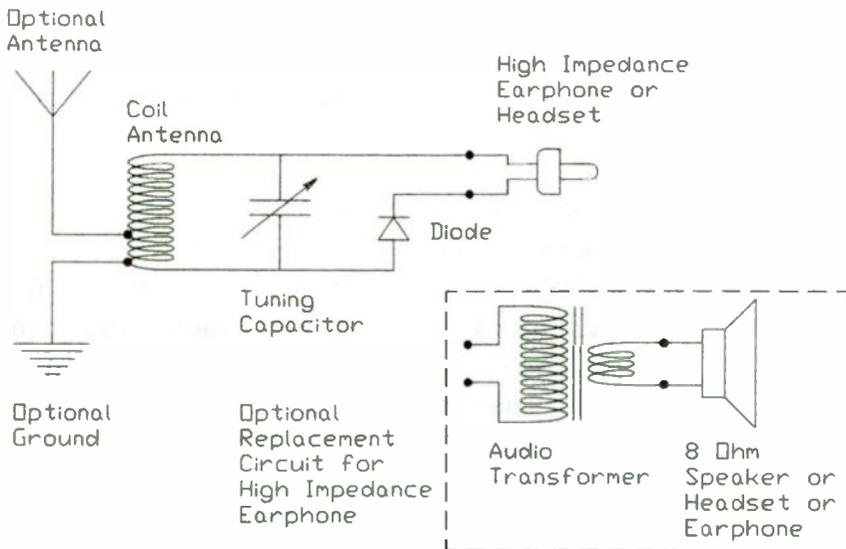
Figure 7: Connection schematic. Note: If a earphone is used rather than headphones, a resistor is required "across" the earphone.
