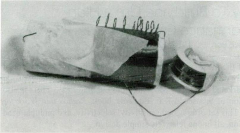
Photo 1: Using tape to hold wire while twisting taps
