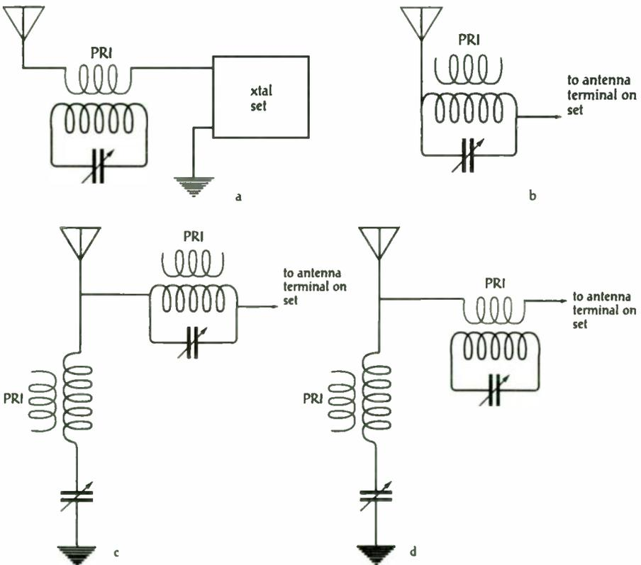
Figure 2: Wave trap schematics (PRI= primary winding)
