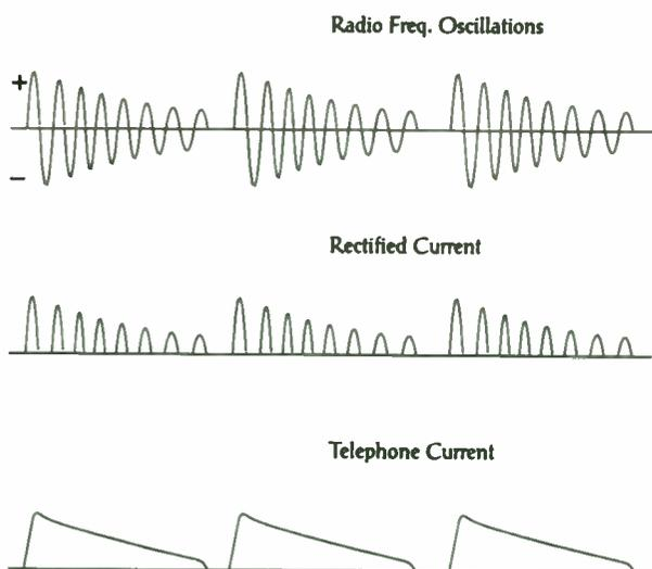
The radio frequency (RF) current, produced by the antenna and the coil, is shown graphically in Figure 3, "Radio Frequency
