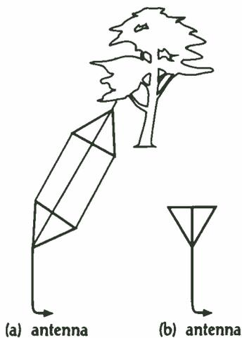
The drawing symbols are often based on the shape or the action of the part they represent. The antenna is no exception. Antennas built by radio pioneers consisted, often, of sets of parallel wires, tied together at a common point (a). The symbol used today is simplified (b). Coils are made by winding wire on a form, typically cylindrical, so the symbol is a spiral (c). Capacitors are made by stacking metal plates, with air or some other non-conducting material between
