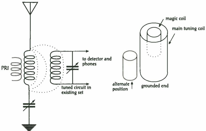
Figure 4: Tuned antenna circuit
