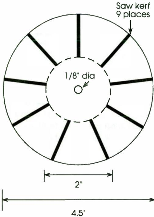
Figure 2: Spiderweb coil form cut from 1/8" plexiglas or lexan
