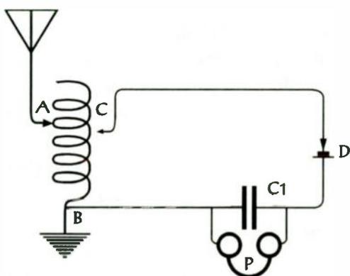
Figure 2: Conductively coupled receiver. A-antenna; B-ground; C-coil; C1-capacitor; D-diode, P-headphones.
