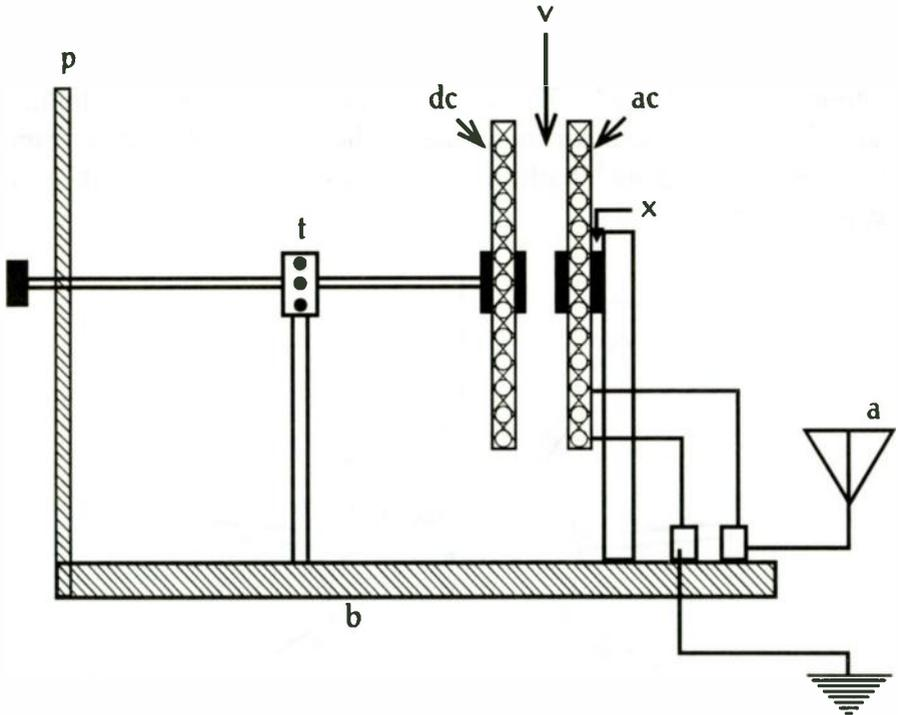
Figure 3: Pictorial diagram of adjustable coil coupling. *P*, panel; *t*, tinkertoy; *dc*, movable detector coil; *v*, variable spacing; *ac*, fixed antenna coil; *x*, plastic piece cemented to coil; *b*, base; *a*, antenna.
