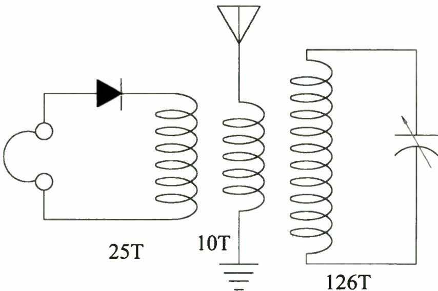
Figure 6: Schematic diagram, detector coil at left, antenna coupling coil center, tuning coil at right.
