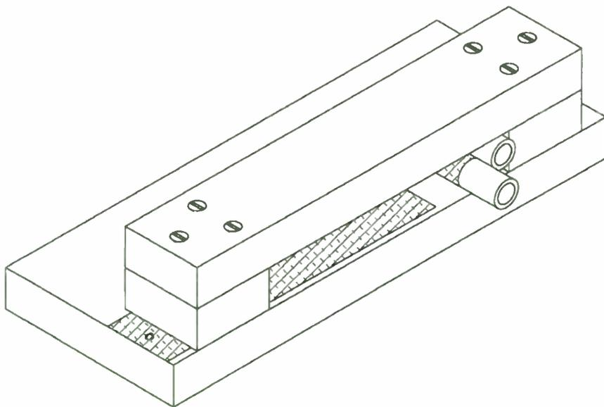
Figure 1: A homemade variable capacitor
