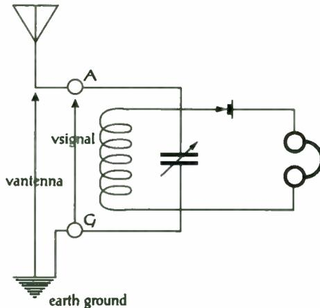
Figure 2: Crystal receiver, non-antenna node of receiver with path to ground
