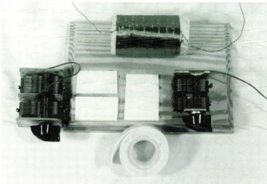
Photo 4: Installing double-sided foam mounting tape prior to securing tuning capacitors
