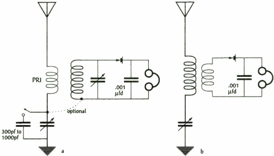
Figure 5: A fixed capacitor in parallel with the variable antenna capacitor
