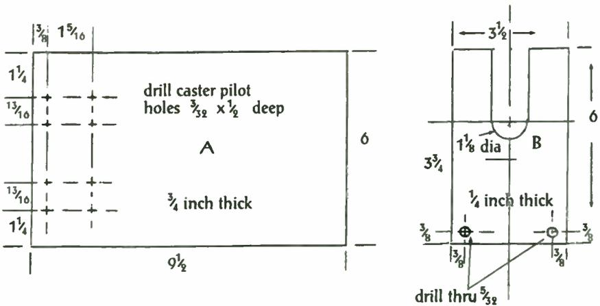
Figure 4: Capacitor assembly and base detail (dimensions in inches)
