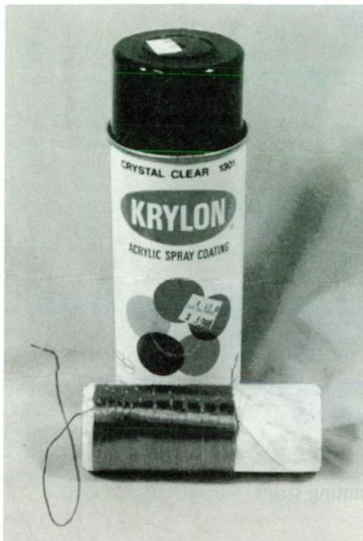
Photo 2: Finished coil before spraying with clear acrylic and trimming coil form
