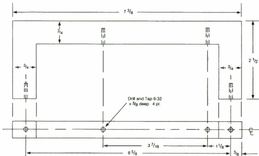
Figure 2: Coil mounting bracket, 1½ inch clear acrylic
