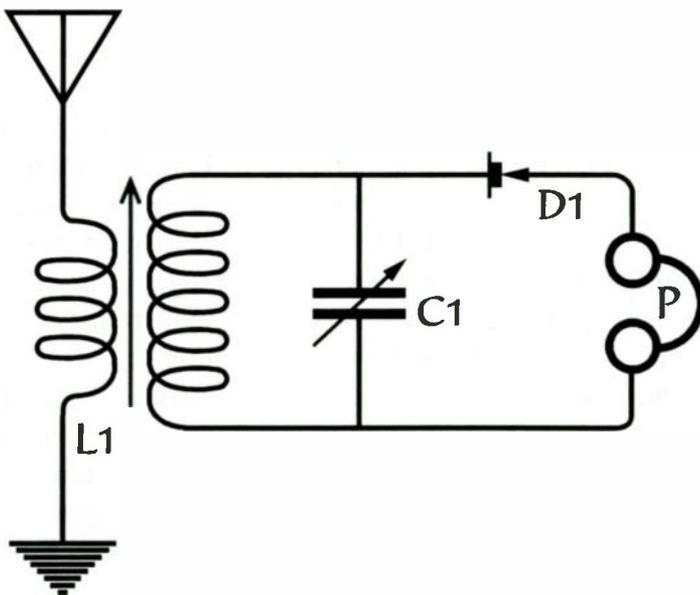
Figure 1: Matchbox crystal radio
