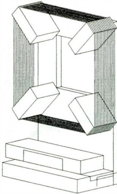
Figure 6: View of frame with wire and tuning capacitor
