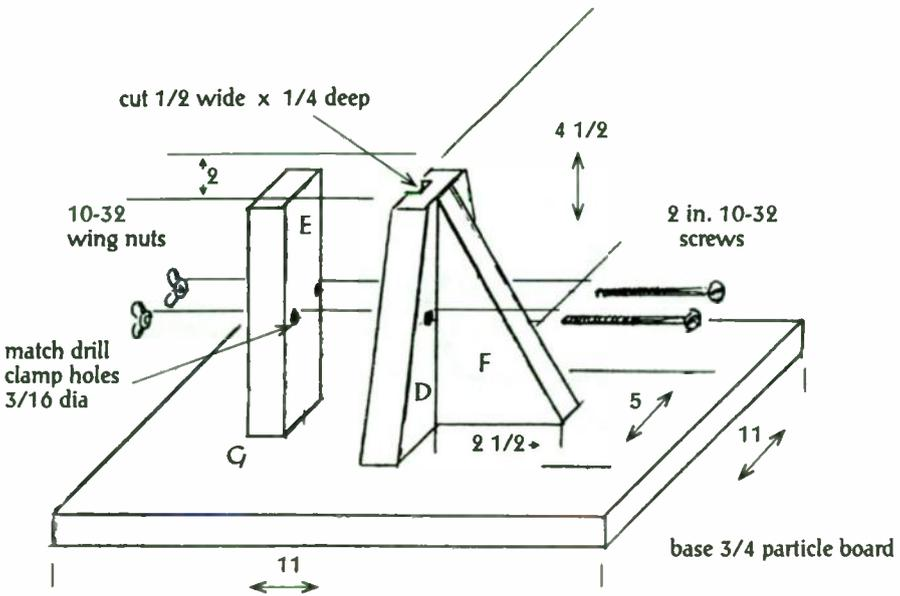
Figure 3: Loop base detail (dimensions in inches)
