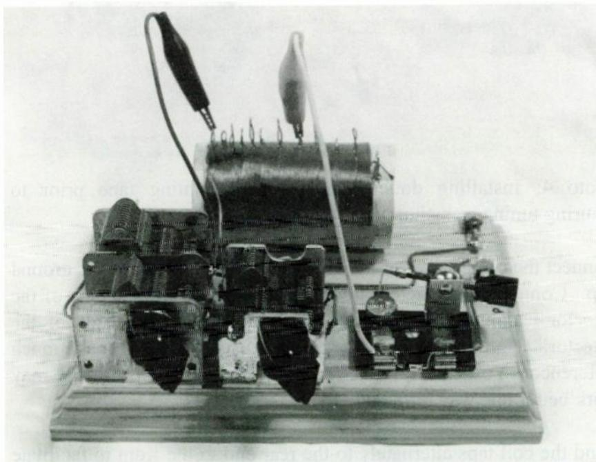
Photo 5: The completed high performance crystal set with 1N34A diode installed in detector clips for testing operation
