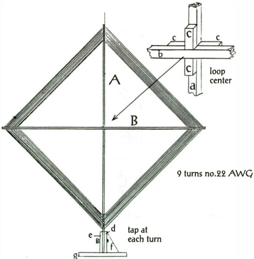
Figure 2: Loop antenna
