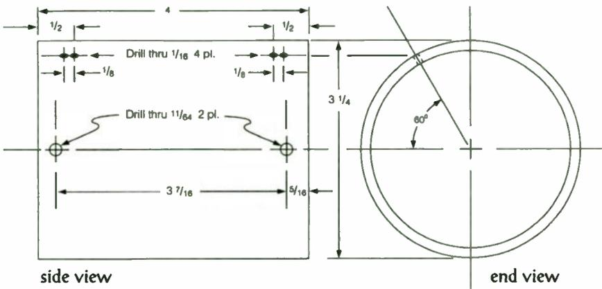
Figure 1: Coil form, 3 inch PVC (dimensions in inches)
