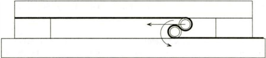
Figure 2: Rolamite bearing capacitor
