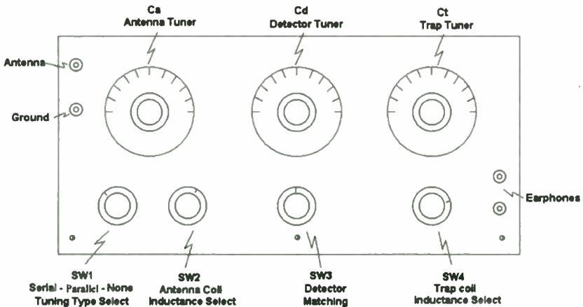
Figure 2: Front panel layout
