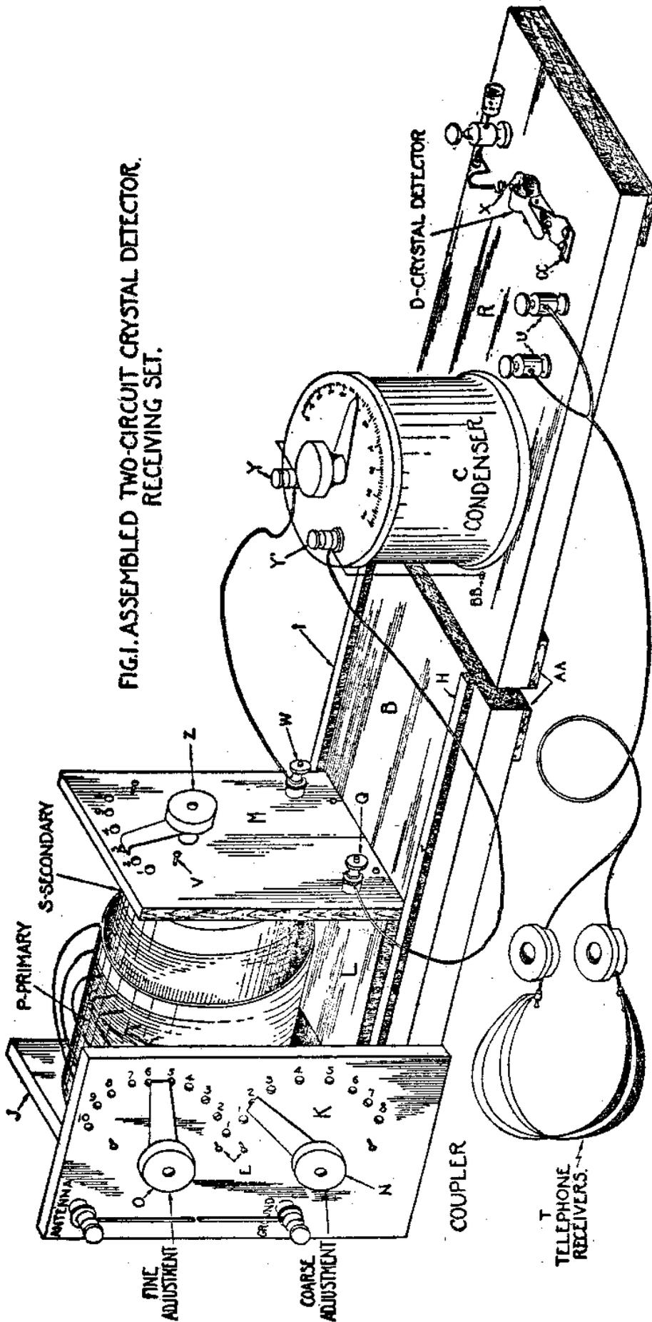
FIG. 1. ASSEMBLED TWO-CIRCUIT CRYSTAL DETECTOR RECEIVING SET.
