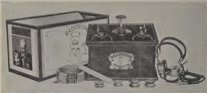
FIG. 49.—The "Radiofone." A loose-coupled type of receiver with stud-switch tuning for aerial inductance, stud-switch inductance-tuning in secondary circuit and variable condenser across latter for fine tuning. Enclosed "permanent" type detector.
