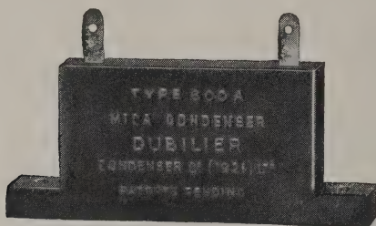
FIG. 73.—A Fixed Condenser composed of Thin Sheets of Copper Foil separated by Sheets of Mica, the whole being imbedded in a special Insulating Compound.
