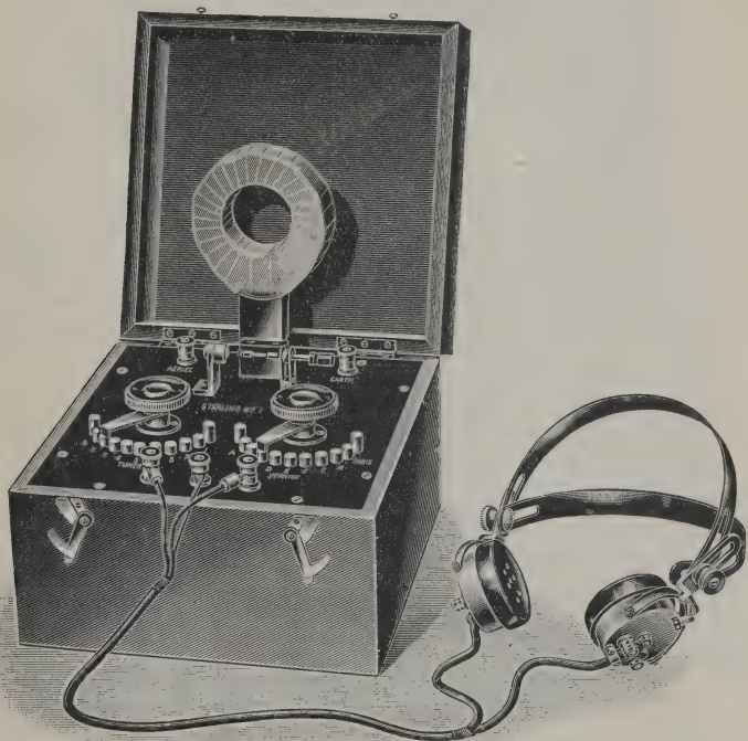
FIG. 23.—The Sterling No. 1 Crystal Receiver. The circuit is that of Fig. 21, with addition of the demountable coil for Eiffel Tower signals.
