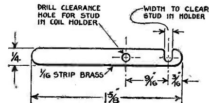
Fig. 85.—Coil-Holder Shorting Switch.
