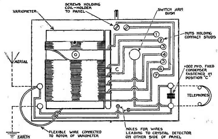
Fig. 76.—View of Back of Panel showing Wiring.
