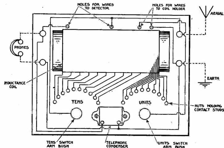
Fig. 90.—Coil Connections.
