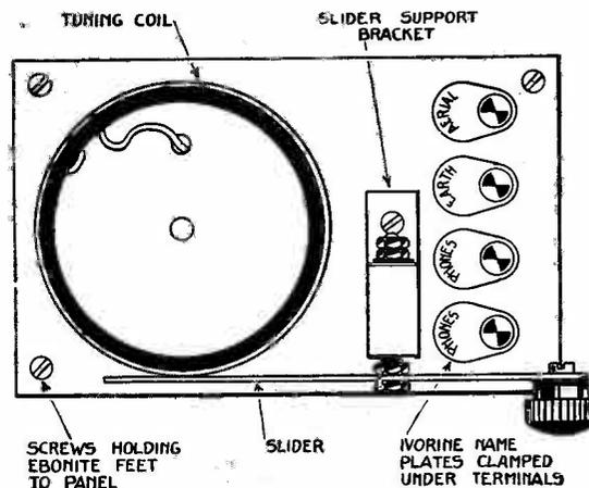
Fig. 28.—Plan of Tuner and Arm.
