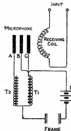
Fig. 55.—Circuit Diagram of "Crystavox."
