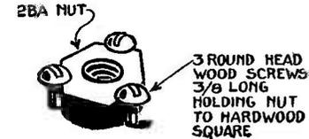
Fig. 22.—Nut for Securing Top Panel.
