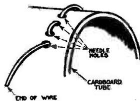
Fig. 97.—Fixing the Wire.
