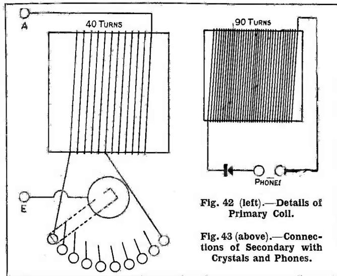
Fig. 42 (left).—Details of Primary Coil.
