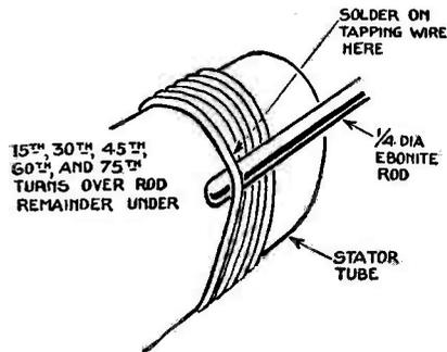
Fig. 71.—Method of Making Raised Wires for Taps.
