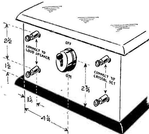
Fig. 137.—Arrangement of Switch and Terminals.
