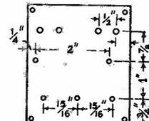
Fig. 16.—Lay-out of Ebonite Panel.
