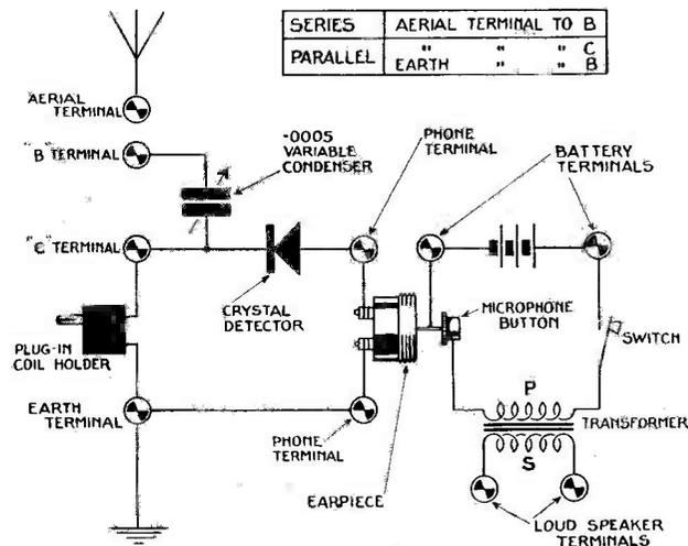
Fig. 129.—Circuit Diagram of Receiver and Amplifier.
