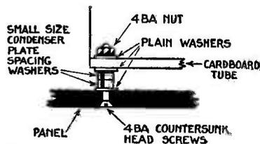
Fig. 83.—Method of Holding Inductance Tube to Panel.
