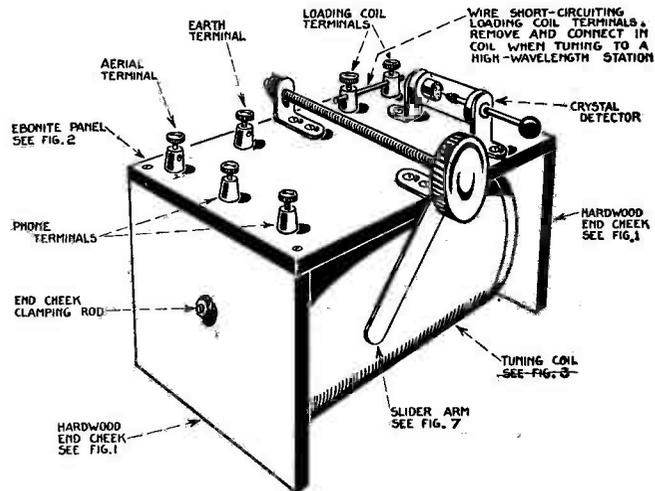
Fig. 99.—Completed Receiver.
