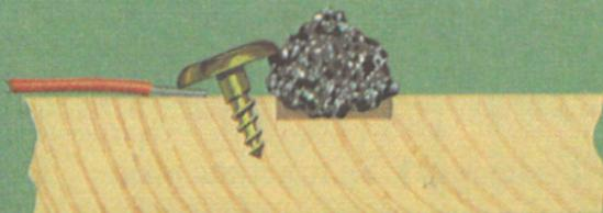
The screw is at a slight angle so as to grip both coke and lead securely
