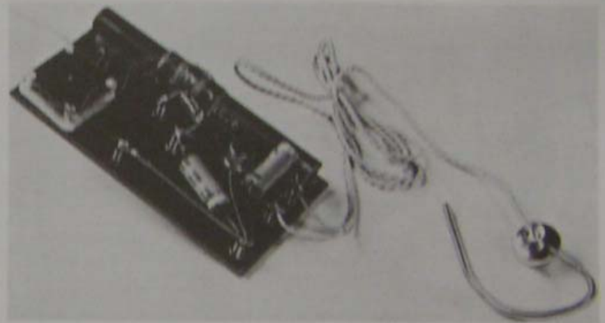
The addition of a capacitor across the phone terminals can improve the quality of reception.
