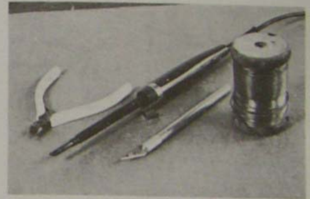
1. The tools you need. Electric soldering iron, cored solder, cutting pliers and a modelling knife.
