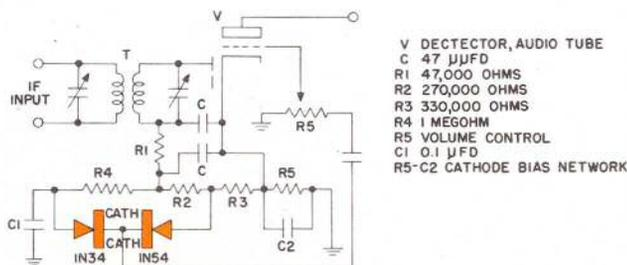
modulation receivers. The circuit is self adjusting to the average level of the received signal, and sharply clips impulse noise components which exceed a certain amplitude relative to it. Using a type 1N54 high reverse resistance crystal as a series clipper element, and a general purpose type 1N34 as a shunt clipper element, this circuit requires few components and little space, yet provides an unusually high degree of impulse noise suppression. • • •
