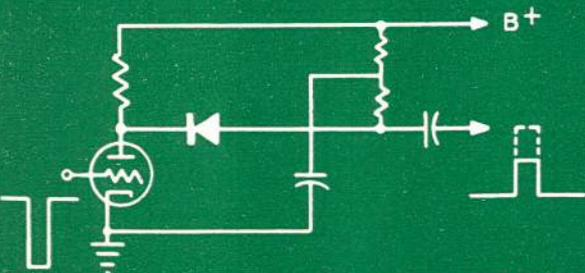
Slicer and video limiter circuits—two of the hundreds of 1N34, 1N38 and 1N39 applications.
