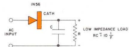
load, with two volts rms applied. Because of its exceptionally low dynamic impedance, the 1N56 provides high current efficiency with load impedances of 1000 ohms and less. Parallel operation of two or more 1N56 crystals will permit correspondingly greater currents to be handled or will increase the current delivered to the load at low input voltage levels.
