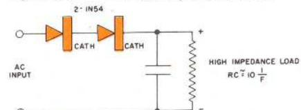
ance upon the efficiency of rectification is substantially reduced by operation of two high reverse resistance type 1N54 units in series. Because the reverse dynamic impedance of the 1N54 reaches a maximum of over two megohms
