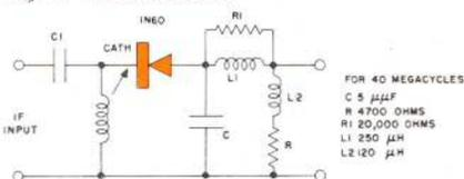
especially designed and tested for this type of service, and provides high circuit efficiency and exceptionally good linearity at low signal levels. Low interelectrode and stray circuit capacitances make for improved video response, and increased overall gain is obtained by virtue of reduced capacitive loading of the detector input circuit. With the component values specified, full 4 megacycle video bandwidth is maintained at the output of the detector. • • •
