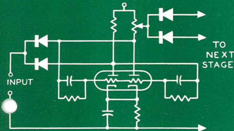
Sylvania germanium crystals are useful as coupling diodes in applications such as this trigger circuit.
