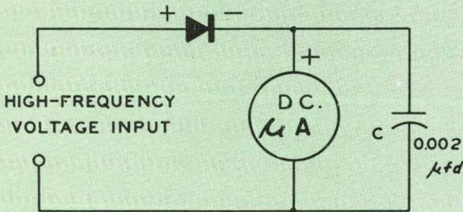
SIMPLE HIGH FREQUENCY, LOW IMPEDANCE VOLTMETER
