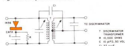
modulation receivers. A high conductance type 1N56, because of its exceptionally low dynamic impedance, provides unusually effective limiting, particularly at signal levels of 5 volts and less. Low diode capacitance produces a minimum of reactive loading across the source, thus minimizing the limiter insertion loss at low levels. • • •
