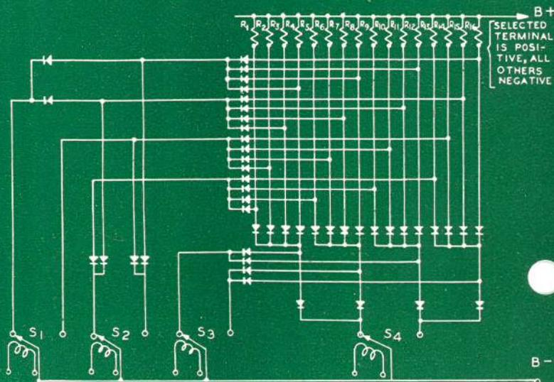
The Crystal Diode Matrix as a high speed selector switch provides another important use for the Sylvania germanium diode family.
