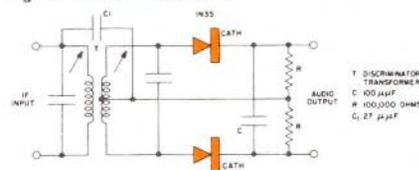
germanium duo-diode, having matched characteristics, provides good circuit balance because of the similar forward conductances of the individual diodes and the complete elimination of contact potential effects. Unusually high diode reverse resistance permits use of load resistance values as high as 100,000 ohms, thus assuring high efficiency, good detector linearity, and low input circuit loading. • • •
