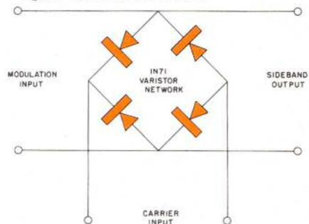
uation obtained with this arrangement is determined by the accuracy of balance within the diode network. Because the 1N71 varistor is made up of four specially selected type 1N56 high conductance crystals whose forward characteristics are closely matched, adequate suppression of undesired carrier components may easily be obtained. In addition, the high conductance features of the 1N71 assure good modulation efficiency because of low network insertion losses. • • •
