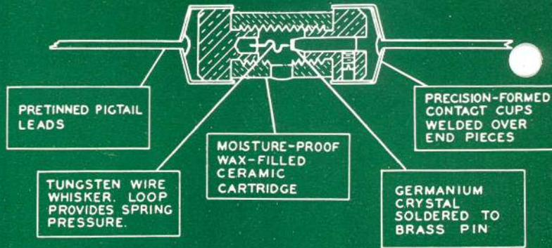
Cross sectional view showing crystal construction details.
