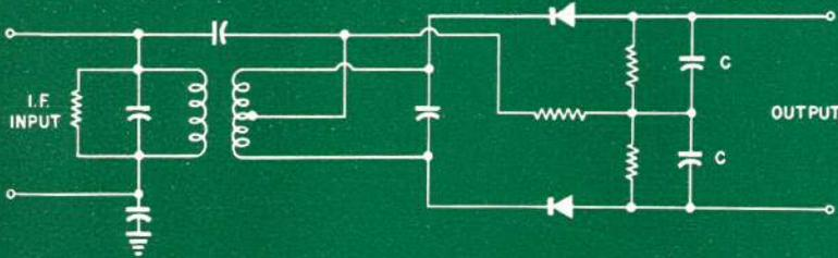
The twin-mounted 1N35 Duo-Diode makes possible a highly compact FM discriminator.
