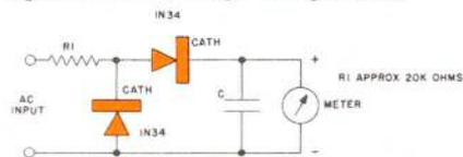
diodes are used in a series-shunt arrangement by which the peak inverse voltage is removed from the series rectifier. A series input limiting resistor acts in conjunction with the shunt crystal to clip off the inverse half of the cycle, thus permitting application of input voltages of peak value up to several times rating of the crystal. The circuit shown in Figure 4 may be useful where a wide range of input voltages must be accommodated. • • •
