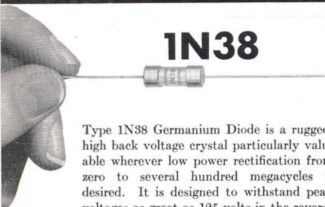
Type 1N38 Germanium Diode is a rugged, high back voltage crystal particularly valuable wherever low power rectification from zero to several hundred megacycles is desired. It is designed to withstand peak voltages as great as 125 volts in the reverse direction. Like the 1N34, its rectification efficiency decreases only 0.07% per degree temperature rise from 27° to 75° C. It weighs less than a penny and can be mounted in any position.
