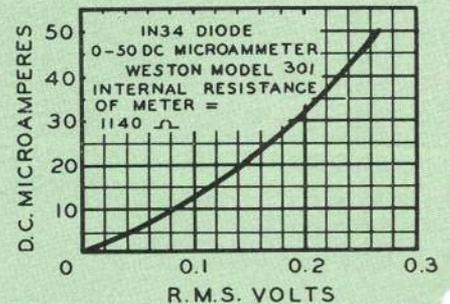
Voltage Calibration Curve for Low-Z Crystal Voltmeter Circuit using a Weston Model 301 0-200 D. C. Microammeter.
