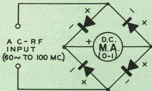
LOW IMPEDANCE, BRIDGE-TYPE A.C. VOLTMETER
