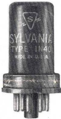
Sylvania Varistors are networks of four carefully selected and matched germanium crystal diodes. They are especially designed for use as ring modulators and bridge circuits in communications modulation and demodulation. They also have applications in many other networks requiring highly polarized non-linear characteristics. Outstanding features are greatly increased frequency range, improved stability, long life and virtual elimination of contact potentials.
