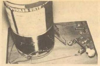
You can't make a simpler, or less expensive BCB receiver than this one. Even the coil winding isn't terribly critical, but the value we selected gave the best result.
