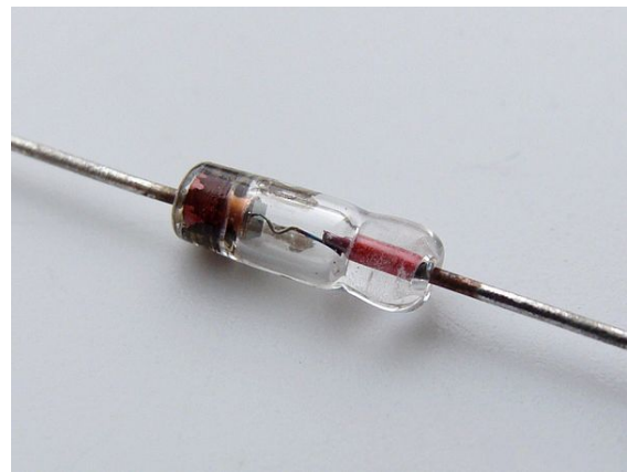
Germanium diode used in modern crystal radios (about 3 mm long)
