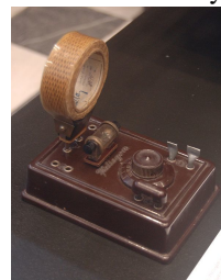
German Heliogen brand radio showing "basket-weave" coil, 1935
