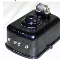
Polish Detefon brand radio, 1930-1939, using a "cartridge" type crystal ( top )
