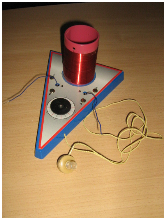
Modern crystal radio with piezoelectric earphone
