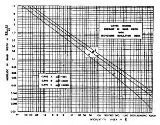
Fig. 5-Variation of bandwidth with modulation index.
