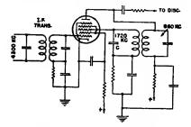
Fig. 2-The locked-in oscillator,
