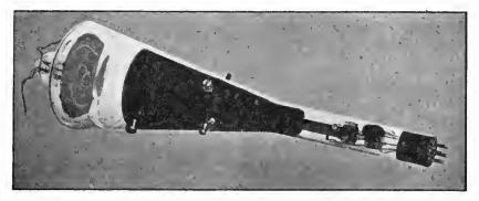
Fig. 5—Early form of the cathode-ray frequency modulation generator, mounted in a standard oscilloscope tube envelope. The target anode is composed of spirals which make one complete turn.
