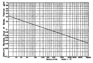
Fig. 3—Absolute maximum value of Bessel function  $J_n(m)$ .
