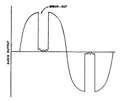
Fig. 7-Breakout characteristic.
