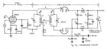
Fig. 8—A ratio-detector circuit using a balanced phase shift transformer feeding a 6AL5 double diode. The closely coupled tertiary winding  $L_{\tau}$  is wound over the  $B^+$  end of the primary to provide impedance matching and improved sensitivity.
