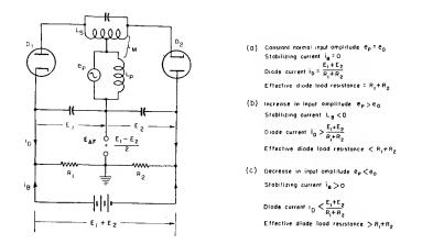
Fig. 6—The effect of changes in input signal level on the diode current, the stabilizing current, and the effective load resistance presented to the diodes. The stabilizing voltage  $E_1 + E_2$  is held constant at the voltage equal to the rectified output when  $e_p = e_0$ .
