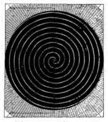
Fig. 8—Spiral anode of five turns, similar to that shown in the tube in Figure 6. The spirals were formed by scribing through a platinum film on a mica support, thus separating the surface into two insulated segments.
