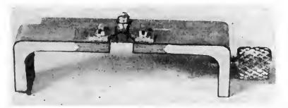
Fig. 10-Push-pull FM plate assembly.
