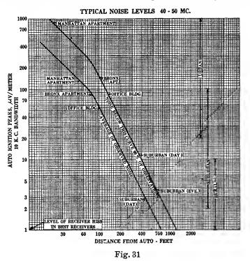
tion shown on Figure 31 is indicative of the noise levels which may be encountered under a wide range of conditions with a 10-kc audio band width. For peak noise the amplitude varies directly with the frequency band. For fluctuation noise the amplitude varies as the square root of the band width.
