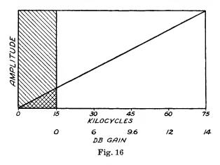
The maximum height of this F-M triangle, corresponding to voltage, is only one-fifth of the height of an FM-15 triangle or the A-M rectangle. Such being the case, the FM-75 advantage over FM-15 is 5 to 1, or 14 db, and over AM it is  $1.73 \times 5$  or 18.75 db.
