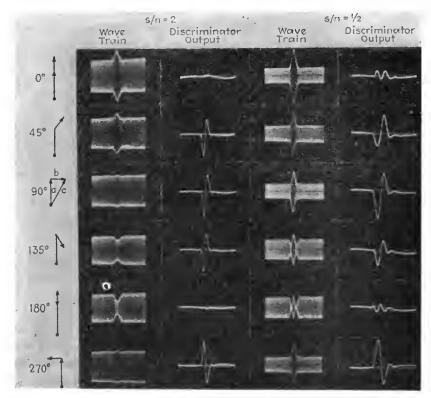
Fig. 3—Right, oscillograms of noise and discriminator output for various phase angles between the noise impulse and signal at two ratios of signalto-noise with the carrier centered in the pass band.
