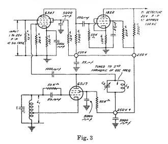
EXPERIMENTAL DETERMINATION OF DETECTOR LINEARITY
