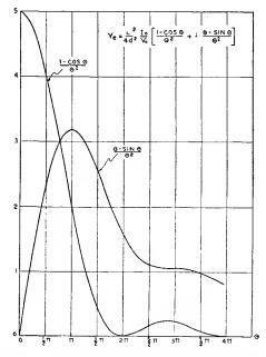
Fig. 2-Electronic admittance as a function of 0.
