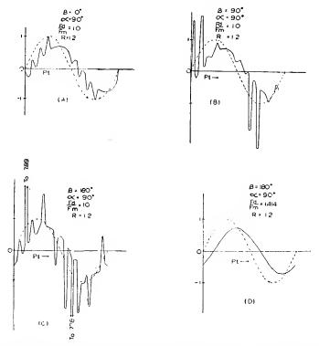
Fig. 8—Calculated wave forms for frequency modulation transmitted over a twopath medium plotted from (6). Ratio between path amplitudes, R = 1.2.  $F_d =$  frequency deviation.  $F_m =$  modulation frequency.  $\alpha =$  phase difference between modulation frequencies.  $\beta =$  phase difference between carrier frequencies. The dotted line curve is a pure sine wave (representing no distortion) for comparison purposes.
