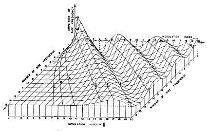
Fig. 4-Side-frequency amplitudes.
