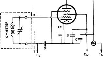
Fig. 2-Circuit for input impedance measurements.
