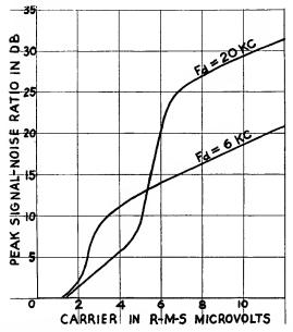
Fig. 1—Peak signal-to-noise ratio characteristics for frequency-modulation systems using maximum frequency deviations,  $F_{d_1}$  of 20 and 6 kilocycles, respectively. The audio band width was 5 kilocycles. The noise was internal receiver noise and the signal-to-noise ratios were measured on an oscilloscope.
