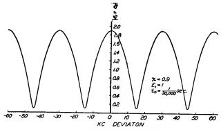
Fig. 7-Variation of amplitude with deviation.
