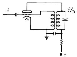
Fig. 10-Locked-In Oscillator Frequency Divider
