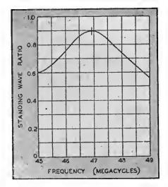
Fig. 15-Standing-wave ratio on the main feed line of a six-layer turnstile.
