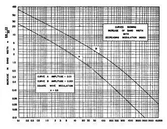
Fig. 11-Variation of bandwidth with modulation index.
