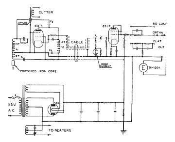
Fig. 13-Schematic of the push-pull FM calibrator.
