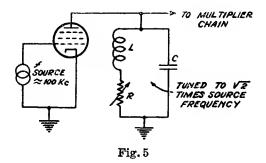
equal in magnitude to the reactance of the circuit capacitance, for all values of R from zero to infinity. Hence, no amplitude modulation is present, regardless of the extent or amount of phase modulation. Appendix I contains a development of the equations of phase vs. R, and also a proof of the constancy of plate-load impedance as R is varied.
