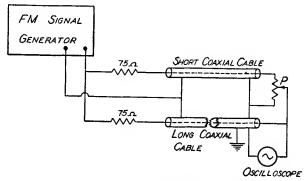
Fig. 8—Circuit for studying interference.
