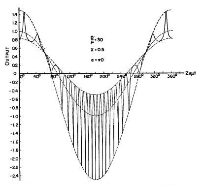
Fig. 19-Common-channel interference, interfering signal detuned.
