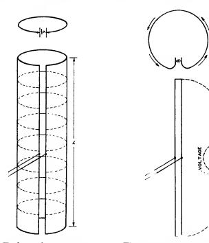
Fig. 3—Each section serves as a number of circular elements.
