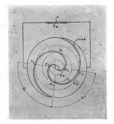
Fig. 2—Typical target anode, consisting of two metal plates divided by a pair of Archimedian spirals. The cathode ray beam scans the target in a circle of variable radius, producing square waves in the output.
