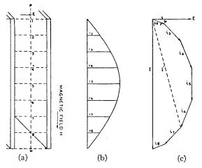
Fig. 3—Vector representation of electron current between parallel plates.
