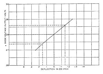
Fig. 7-Linearity of the push-pull FM system (distortion).
