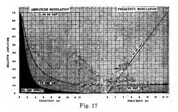
program modulation, depending upon the character of the sound source. The NBC field test confirmed these conclusions. Therefore, in presetting transmitter gain controls, using low-frequency tone modulation, a 2.5 db correction should be made for program modulation.
