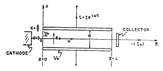
Fig. 1-Schematic diagram of beam and electrode arrangement.
