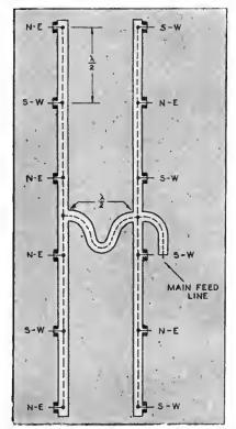
Fig. 9-A practical feed system for six layers or more.
