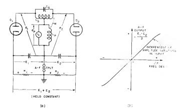
Fig. 2—Basic circuit of a ratio detector using the same phase shift input circuit as in Figure 1. The rectified voltage is stabilized so that the output can be independent of the input amplitude.
