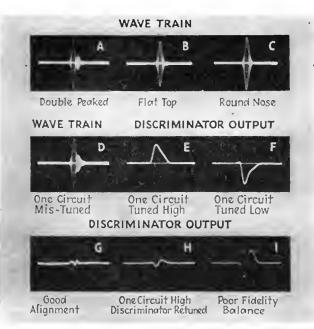
Fig. 1—Oscillograms of noise wave train and output of discriminator for various conditions of tuning.
