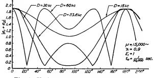
Fig. 4-Variation of carrier envelope with D.
