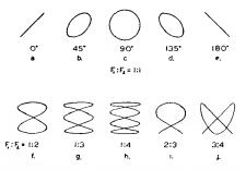
Fig. 5—Lissajou figures obtained with various phase relations and frequency ratios between voltages applied to opposite oscilloscope plates.
