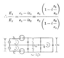
Fig. 20—The ratio-detector circuit in a more general form. The voltages  $e_1$  and  $e_2$  may be produced in various ways, including the phase-shift circuit and side-tuned circuits.
