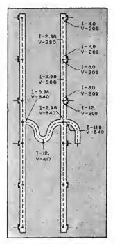
Fig. 16—Voltage and currents on the feed lines of a six-layer turnstile, operating with a power of 10,000 watts.
