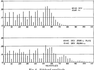
Fig. 6-Sideband amplitude.
