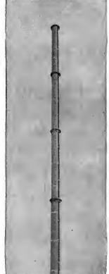
Fig. 2—A 4-section pylon antenna, mounted on the roof of a building.
