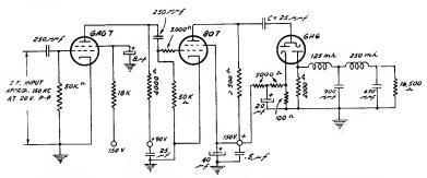
Fig. 2-90-volt and 150-volt supplies are regulated. One side of all heaters (supplied from 6.3-volt transformer) is grounded.
