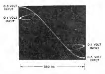
Fig. 11—Effect of reduction in the input signal. The stabilizing voltage is held constant at a level corresponding to the 0.3-volt input signal. Note the reduction in peak separation for decreasing input signal.
