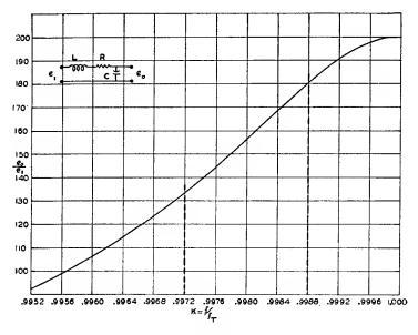
Fig. 8-One side of the discriminator resonance curve.
