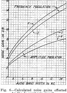
by the de-emphasis circuit. Curves F = fluctuation noise. Curves I = impulse noise.
