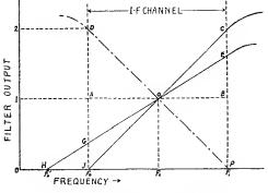
Fig. 2-Ideal sloping filter characteristics.
