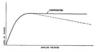
Fig. 12-Effect of signal voltage on lock-in range.
