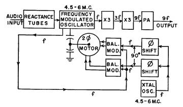
Fig. 7-Preliminary Frequency Control FM Exciter
