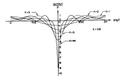
Fig. 12-Effect of low-pass filter.
