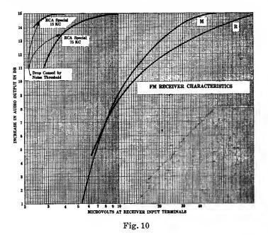
voltages. The drop in the field test receiver is due to the noise threshold limitation and not lack of r-f gain.
