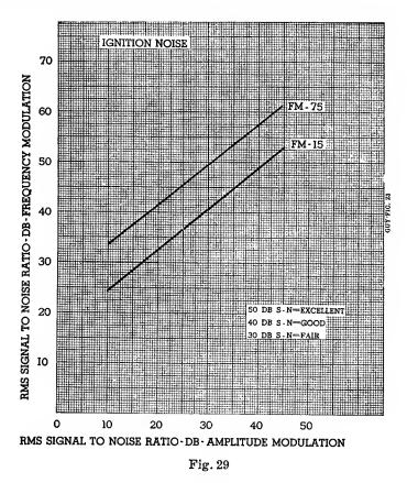
the system made the accuracy of S/N measurements in the 60-db region uncertain. Of particular interest is the shape of the F-M curves at the lower right side of the figure. The explanation for it is given in the references.
