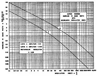
Fig. 12-Variation of bandwidth with modulation index.
