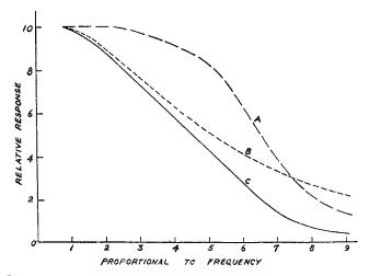
Fig. 4-Frequency-response curves of wide-range frequency discriminator.
