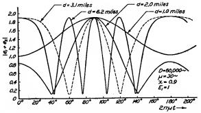
Fig. 6-Variation of carrier envelope with path difference.
