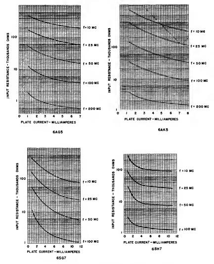
Fig. 4-Input resistance variation with plate current.
