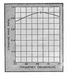
Fig. 14-Standing-wave ratio on the main feed line of a four-layer turnstile.
