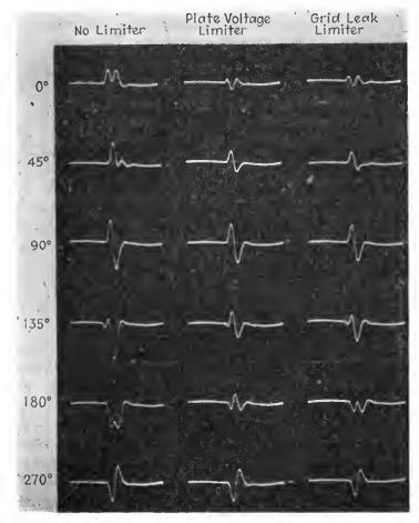
Fig. 7—Oscillograms illustrating noise reduction by plate voltage and grid leak limiters.
