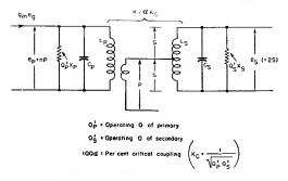
Fig. 15—A further simplification of the equivalent circuit of Figure 14, showing the voltages P and S which are applied to the rectifier circuit.
