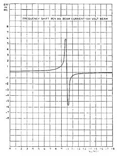
Fig. 13—Frequency shift versus magnetic field for the rectangular cavity structure.
