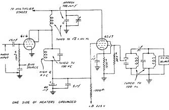
Fig. 8-Phase modulator circuit.
