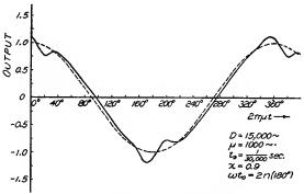
Fig. 22-Distorted audio output.
