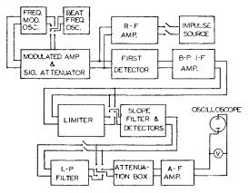
Fig. 7-Block diagram of experimental setup.
