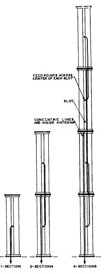
Fig. 5-Feeder system used for 1, 2, and 4 sections is exceedingly simple.
