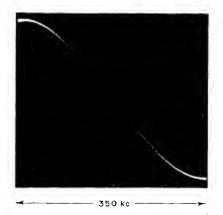
Fig. 10—Output characteristic and performance data for the ratio detector shown in Figure 8. Input signal = 100 millivolts; Rectified voltage = 6 volts; A-V-C voltage = 2.5 volts; A-F output (75-kilocycle deviation) = 0.7 volt root-mean-square; Distortion (100 per cent modulation) = 2.5 per cent root-mean-square; Distortion (30 per cent modulation) = 0.7 per cent rootmean-square; Maximum downward amplitude modulation = 70 per cent.
