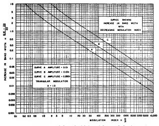
Fig. 17-Variation of bandwidth with modulation index.
