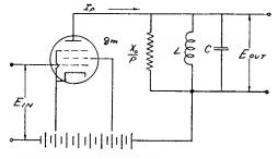
Fig. 3-Simplified schematic of a tuned amplifier.
