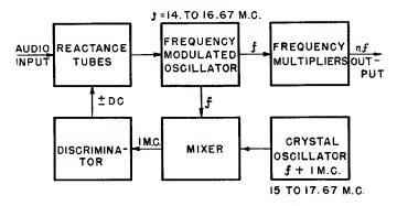
Fig. 4-Reactance Tube FM Exciter.
