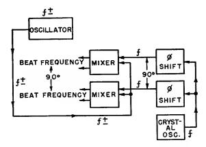
Fig. 6-Fundamental Frequency Control Circuit
