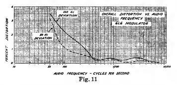
The distortion at high audio frequencies is independent of modulator bias, but is very much a function of tuning, even with sufficient circuit damping. This is particularly the case in the 300-kc tripler following the mixer stage, which must accommodate a band of frequencies 15 times as great as that encountered in circuits directly following the modulator.
