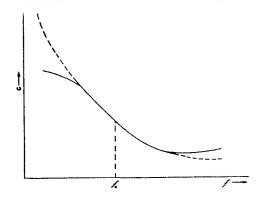
Fig. 11-Matching the discriminator to the oscillator.
