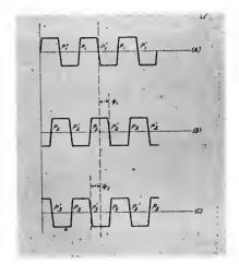
Fig. 4—Square wave outputs of the generator, lettered to correspond with the scanning circles shown in Fig. 2, opposite. The phase shift results in frequency modulated waves when the signal is passed through a frequency multiplier.
