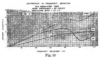
$E_{g}$  curve. This can be corrected, if desired, by some types of regenerative audio circuits, which tend to increase non-linearity in the modulator tube  $R_{p}$  curve, or by the use of an additional modulator to supply 2nd harmonic variations in  $R_{p}$  to produce additional curvature.
