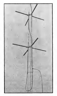
Fig. 7—Individual layers are connected together by means of two concentric lines which spiral around the pole. A simple matching network is also shown.
