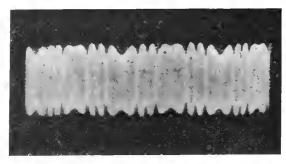
Fig. 10-Oscillogram of carrier envelope.
