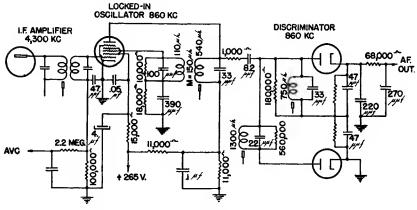
Fig. 16-Locked-in oscillator and discriminator.
