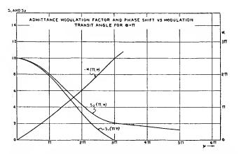
Fig. 8—Admittance modulation factor and phase shift ve.sus modulation transit angle for  $\theta = \pi$ .
