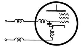
Fig. 3a-Series resonance in tube input circuit.
