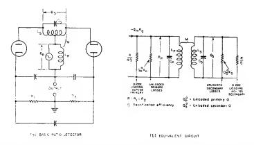
Fig. 13—The equivalent circuit for a basic phase shift ratio detector show. that the diodes reflect an equivalent shunt resistance  $R/4\eta$  across the primary and a resistance  $R/\eta$  across the secondary.
