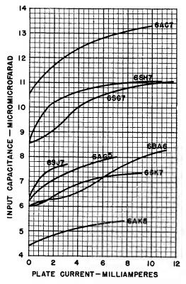
Fig. 7-Input capacitance variation with plate current.
