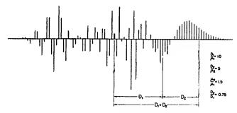
Fig. 6-Spectrum for complex modulation.
