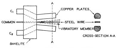
Fig. 6-One form of push-pull FM transducer.
