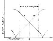
Fig. 3—Characteristics of the conversion filters used to convert frequency modulation into amplitude modulation for detection.
