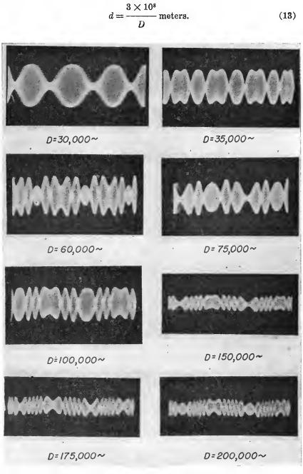
Fig. 9-Oscillograms of carrier envelopes.
