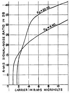
Fig. 2—Root-mean-square signal-to-noise ratio characteristics for the same systems used for Fig. 1. The signal-to-noise ratios were measured on a rectifier-type meter.
