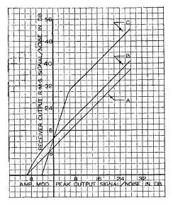
Fig. 10—Measured root-mean-square signal-noise ratio characteristics for fluctuation noise. Curve A = amplitude modulation receiver. Curve B = frequency modulation receiver with deviation ratio equal to unity. Curve C = frequency modulation receiver with deviation ratio equal to four.
