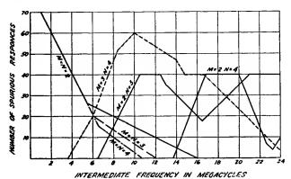
Fig. 1—Spurious responses caused by harmonic combinations of signal and oscillator versus intermediate frequency. Signals: from 40 channels between 42 and 50 megacycles. Tuning: from 42 to 50 megacycles. M = signal-harmonic order.
