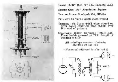
Fig. 9—Details of construction of the ratio-detector transformer used in the circuit of Figure 8. The bifilar secondary connections are brought out symmetrically to the vertical rods to prevent unbalance.
