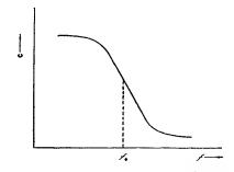
Fig. 9-Input capacitance of discriminator.
