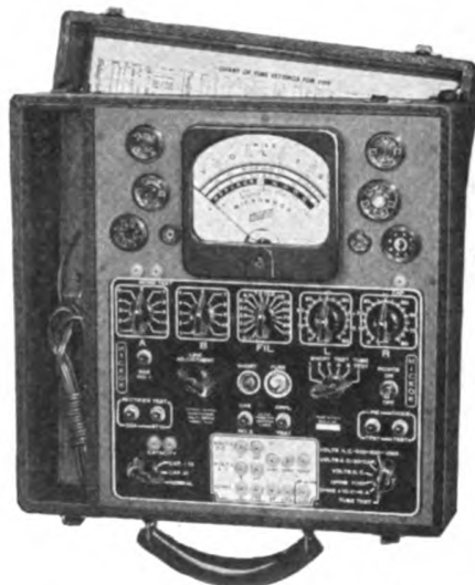
Figure 263. A dynamic tube tester which will detect all possible faults in vacuum tubes.
