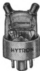
Figure 213. For high frequency oscillators, special vacuum tubes, having very small inter-electrode capacity, are employed.
