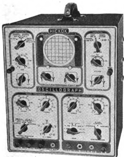
Figure 281. Most oscilloscopes employ three inch cathode ray tubes and have the required controls for adjustment to "see" signals of various types.
