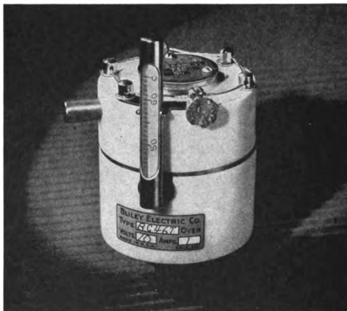
Figure 219. To eliminate variations due to temperature, specially constructed thermostatically controlled ovens are employed. The temperature inside the oven is kept at a constant value.
