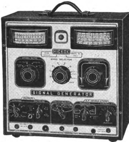
Courtesy Hickok Electrical Inst. Co. Figure 276. A good quality R.F. signal generator incorporating a decibel meter for measuring the output signal level of a radio receiver.
