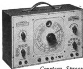
Figure 275. A condenser tester employing a bridge circuit is a handy instrument for the laboratory or the more advanced radio shop.
