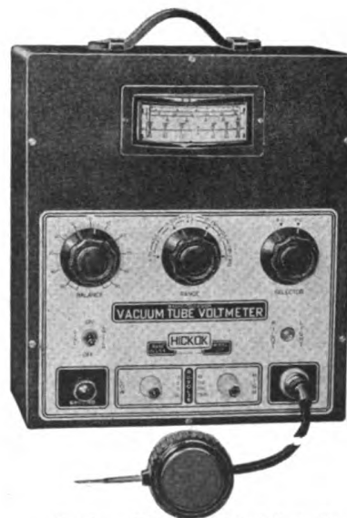
Figure 279. A vacuum tube voltmeter incorporating a type 955 acorn tube in the probe to reduce the input inter-electrode capacity. Notice that the dial at the left is used for zero adjustment, the center dial for range selection, and the right hand knob for adjusting the circuit for either D.C. or A.C. operation.
