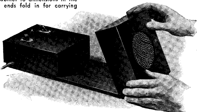
Make the wooden cabinet to dimensions in the drawing. Note how ends fold in for carrying
