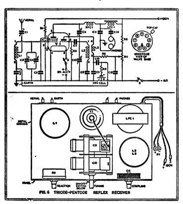
to-vay, and any method by which parts could be dispensed with was considered a major advantage. In a reflex receiver, one valve is made to perform the duty of two or more by shunting the signal round the circuit. by-passing any unwanted portion and returning it to its point of entry for yet further amplification. This system is not to be confused with the more orthodox process of using, perhaps, a double triode in a straight circuit one half as a detector and the other half as an amplifier.
