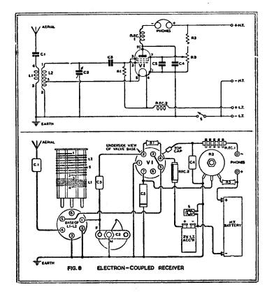
panel of metal. V1 should be mounted horizontally to avoid having the anode lead unnecessarily long. The coils L1-2 are best wound on 6-pin formers, obtainable from any supplier dealing with short-wave components, complete with sockets to fit. Eddystone-threaded formers were used on the original. Three coils are usually sufficient to cover the popular bands, and the table gives the required turns and wave-band covered.
