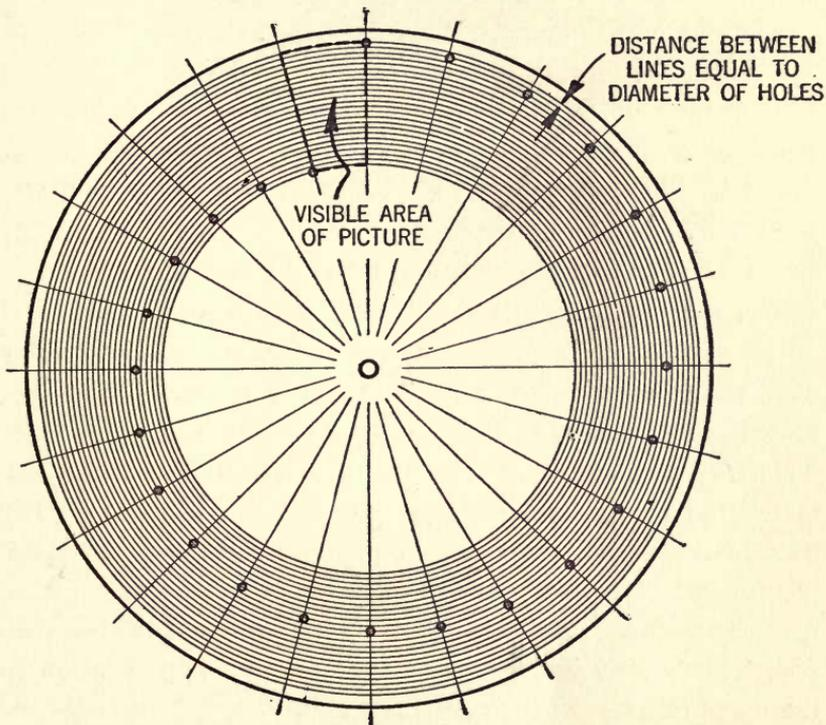
FIG. 53.—Simple way of laying out a television scanning disc for drilling. By this method the spiral automatically develops, its formation requiring no elaborate measuring instrument or involved formula.
