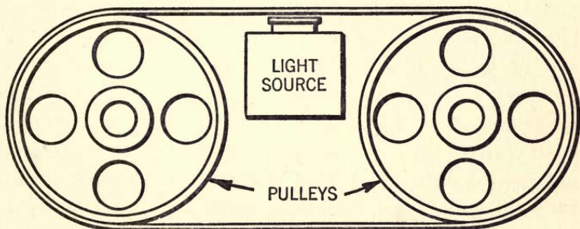
FIG. 55.—How scanning may be provided with a belt. The holes, in place of being drilled in spiral fashion, are simply drilled along the line of an angle.
