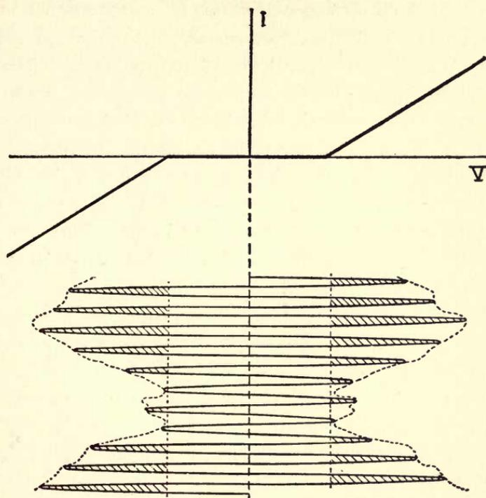
FIG. 41.—Diagrammatic representation of the relation between modulated high frequency wave impressed on grid type neon lamp and lamp characteristics. The intensity of the glow is proportional to the shaded area. (Courtesy Bell Telephone Laboratories, Inc.)
