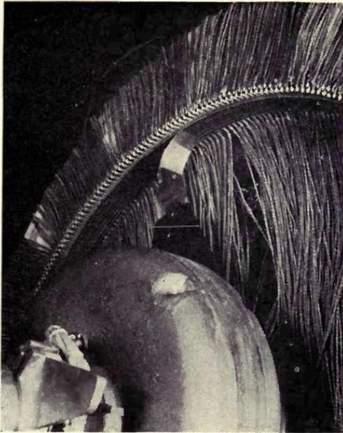
Here is a part of the 2500 separate wires running from the contacting device to the 2500 tinfoil electrodes on the large neon tube of the Bell Telephone television system. The revolving contactor connects each one of the electrodes once during each revolution. Naturally, this revolving arm runs in synchronism with the scanning device at the transmitter. (Photo Courtesy Bell Telephone Laboratories, Inc.)
