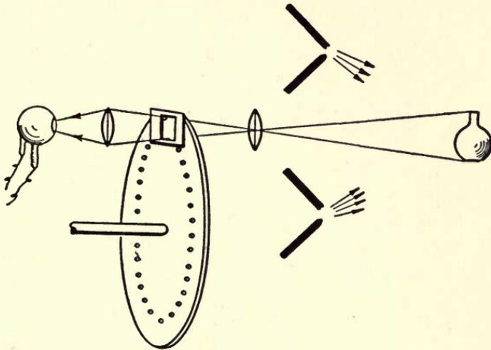
FIG. 62.—In this scanning system, the object to be transmitted is illuminated with several powerful sources of light. (Courtesy Bell Telephone Laboratories, Inc.)
