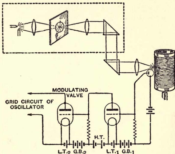
FIG. 6.—Showing the arrangement of the essential parts of the Karolus picture transmitter. The photoelectric cell is shown mounted adjacent to the picture on the revolving cylinder.
