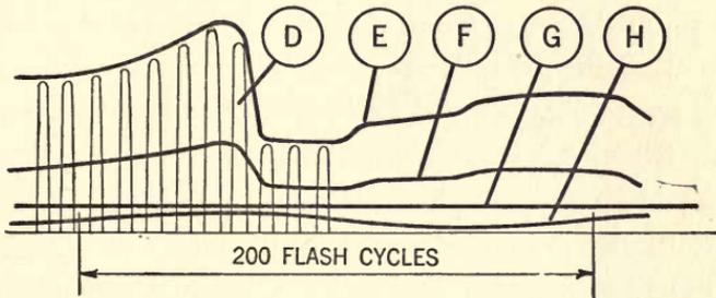
FIG. 72.—D. Neon lamp flashes, 40,000 per second. E. Flash energy applied to delineate picture on screen. F. Energy reflected by the small fixed mirror, Fig. 1, to fall upon the chopper. G. Maximum illumination required on the photoelectric cell to compensate for one per cent slow speed. H. Approximate synchronizing cycle made up of 200 flashes.
