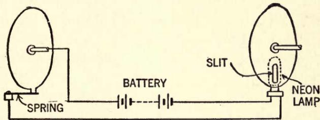
FIG. 69.—Simple indicator of synchronism. When the glow of the neon lamp is seen, this indicates that the wheel at the transmitter is running in perfect step with the wheel at the receiver.
