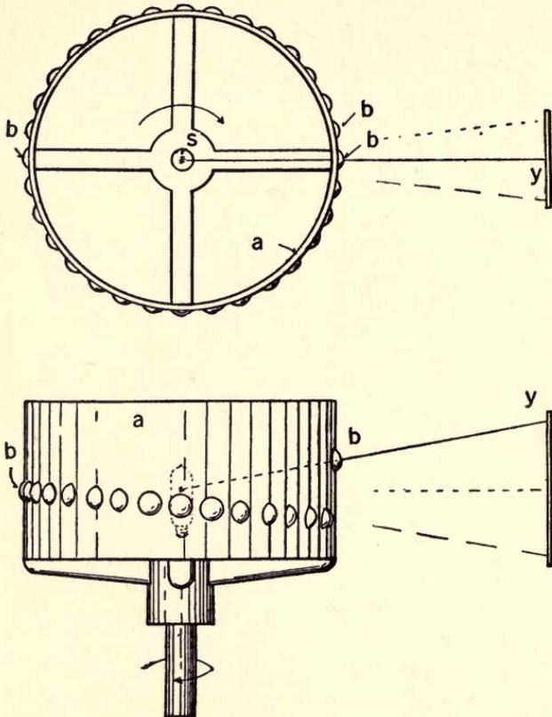
FIG. 61.—Jenkin's method of employing a drum for scanning. The lenses are mounted in spiral fashion.
