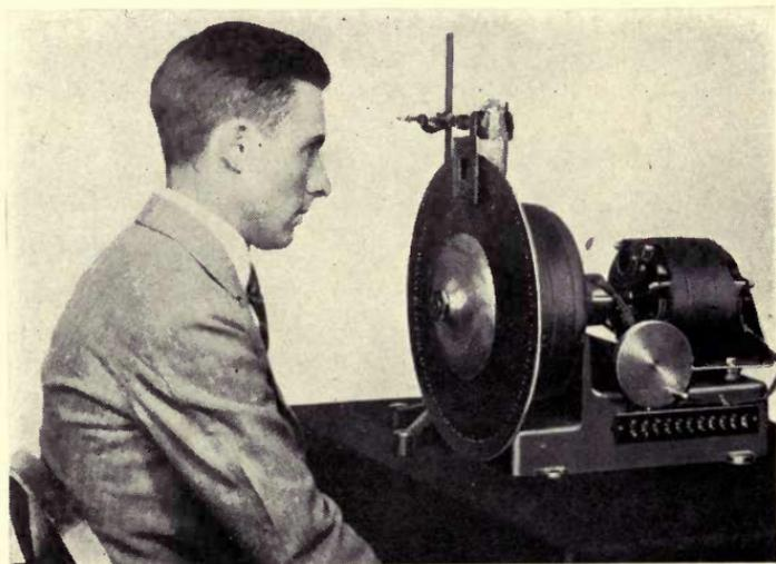
An observer sitting before a television receiver. The picture appears in the small square aperture, the neon tube being mounted directly in line with this member. Two driving motors are used in this system, one a 60-cycle synchronous motor and one a 2000-cycle synchronous motor. (Courtesy Bell Telephone Laboratories, Inc.)
