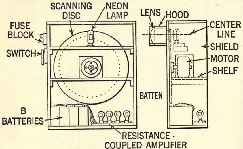
FIG. 78.—General arrangement of the parts making up a television receiver. The box is made of three-quarter-inch white pine painted black inside to prevent reflection and to sharpen the outline of the received picture.
