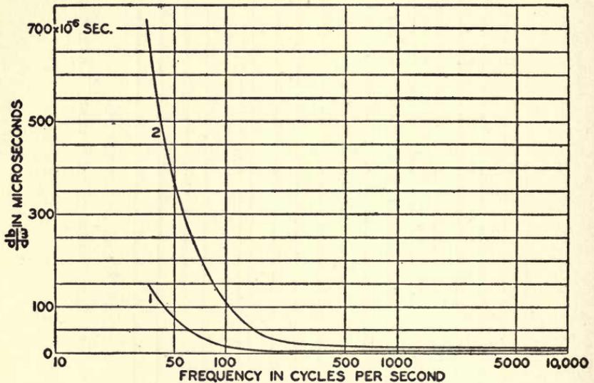
FIG. 37.—Envelope delay characteristics of (1) an output transformer and (2) a high-ratio input transformer. (Courtesy Bell Telephone Laboratories, Inc.)
