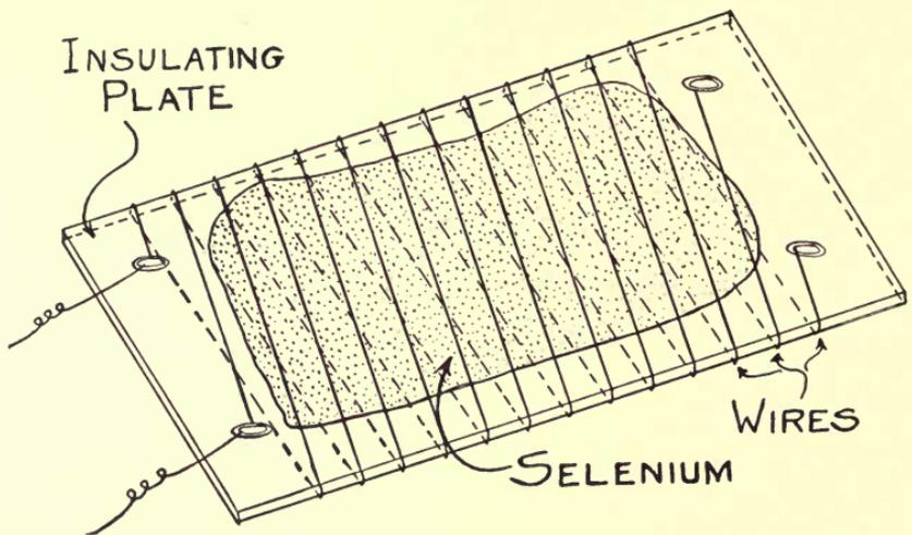
FIG. 2—Construction of an early type of selenium cell.
