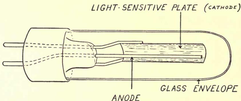
FIG. 3—Construction of a photoelectric cell.
