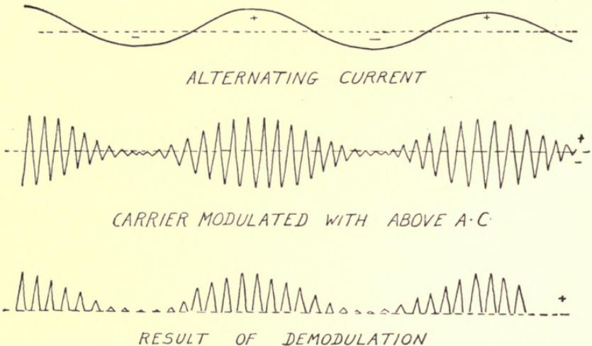
FIG. 24—Amplitude modulation of a carrier current.
