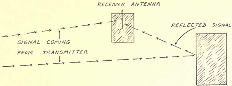
FIG. 48—Diagram showing double signal reception by an antenna; one signal coming direct from the transmitter, the other being reflected from a tall building behind the home of the viewer.
