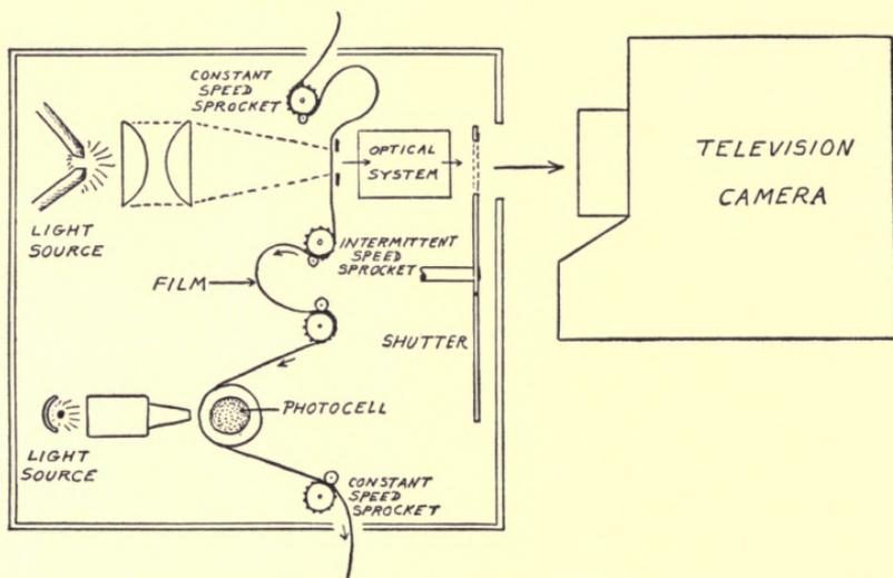
FIG. 40—Use of a film-scanner in converting motion picture scenes into television images. The motion picture projector is outlined in section view at the left.
