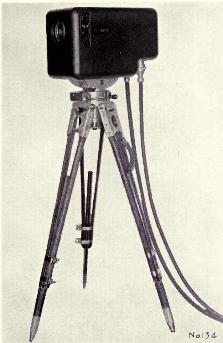
Fig. 13. The Farnsworth Pick-Up Camera complete. (Note compactness)
