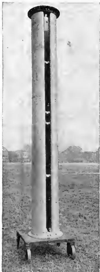
Fig. 1—Single pylon antenna section.
