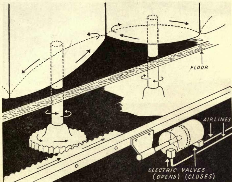
MECHANICAL DEVICE WHICH CONTROLS ACOUSTIVANES
