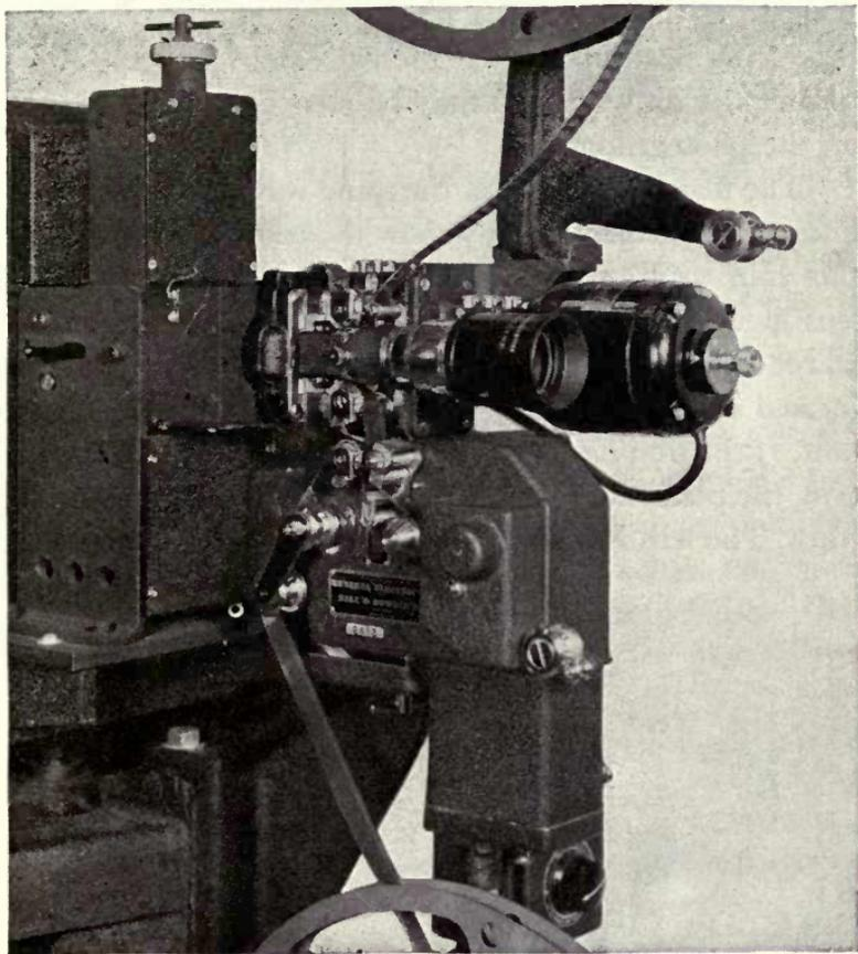
Fig. 4-15. Close-up of GE 16 mm projector mechanism.
