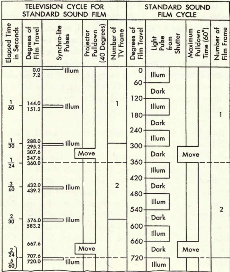
Fig. 4-6. GE synchronizing cycle for film projector operation over television.
