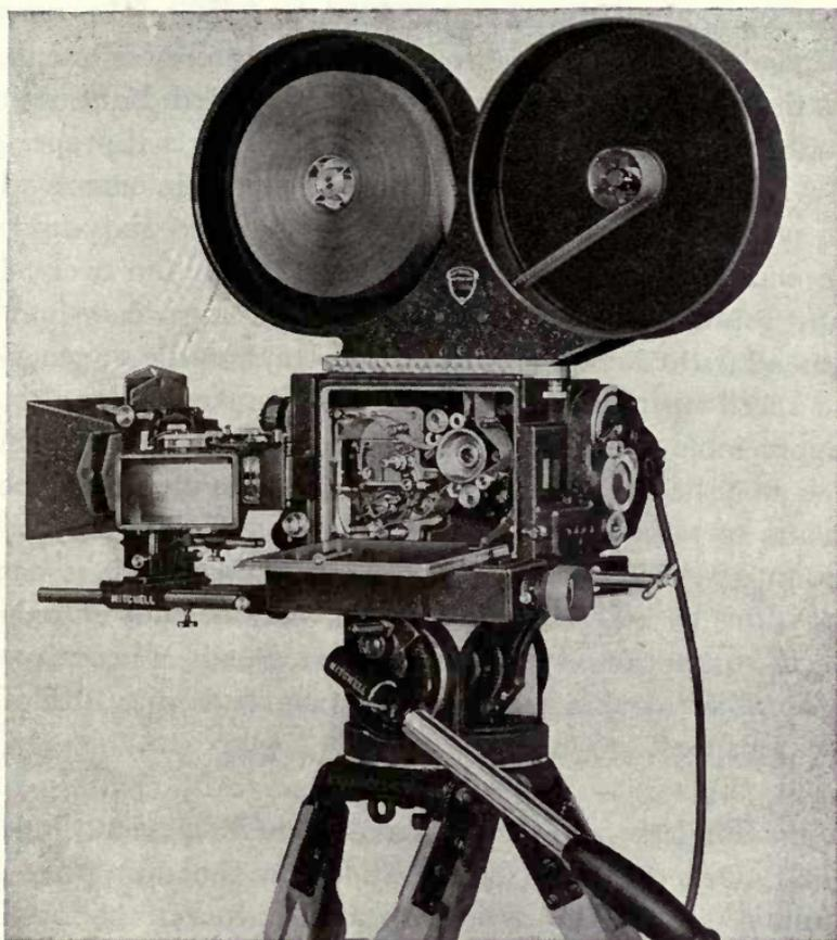
Fig. 3-12. Opened view of Mitchell 35 mm sound camera. The heavy construction and solid workmanship of this fully professional Hollywood camera are very apparent.
