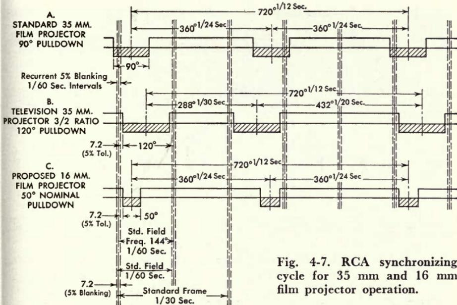
Fig. 4-7. RCA synchronizing cycle for 35 mm and 16 mm film projector operation.
