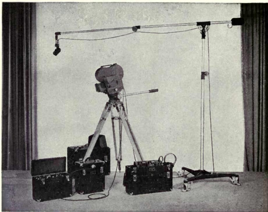
Fig. 3-4. Group of Auricon camera and sound equipment.
