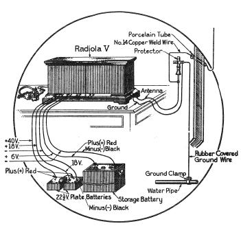
receiver as possible. When using Radiotron UV-200 as a detector, make the battery and other connections as indicated on the diagram. When Radiotron UV-201 is used as a detector, omit the lead from the 18-volt terminal of the battery and connect together the "+18 V." and "+40 V." terminals on the rear of the receiver.
