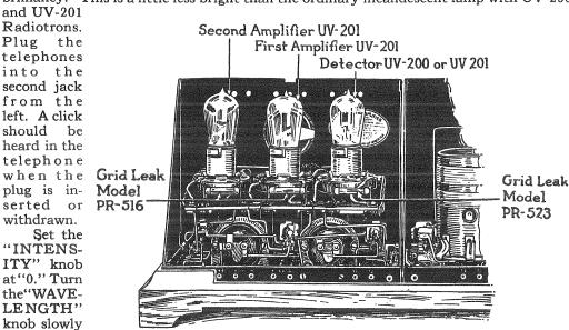
until a signal is heard, and leave it at the point where the signal is loudest. If no signals are heard, or if they are very weak, slowly turn the "INTENSITY" knob clockwise, still searching for signals with the "WAVELENGTH" knob.
