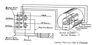
8-60 Input Transformer Wiring
