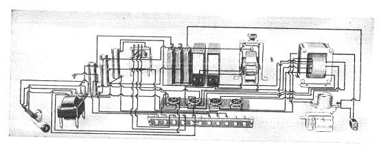
Parts and Wiring of Power-Amplifier Unit AP 997 (RPA 5 Special) (Used in 8-60)
