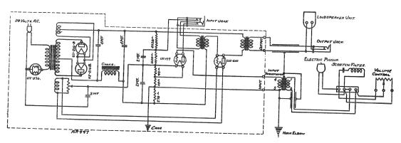
Wiring Diagram for Electrola 8-60
