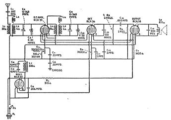
Figure A—Schematic Circuit
