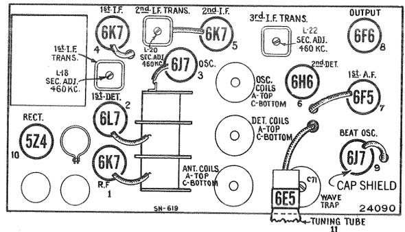
Figure 10—Radiotron and Coil Locations.
