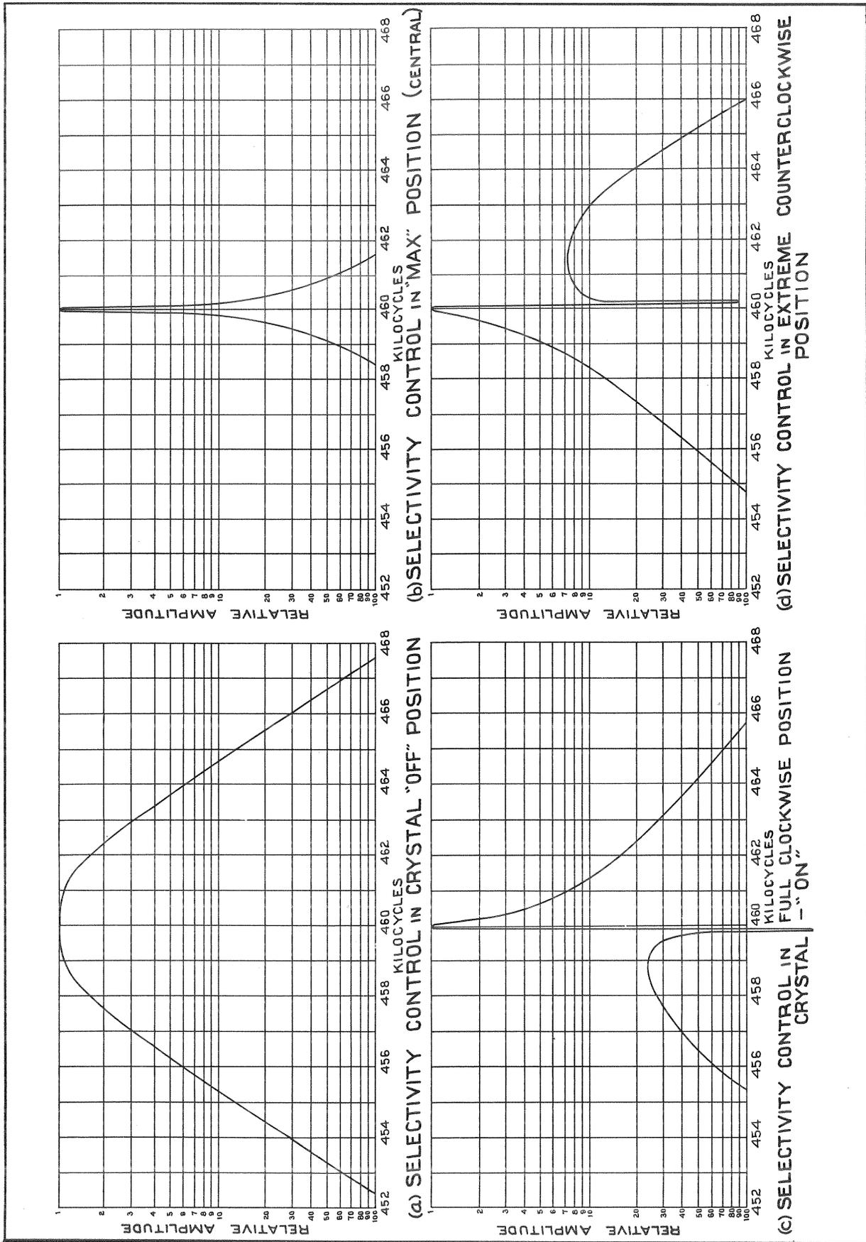
Figure 5—Selectivity Control Curves.—Crystal Filter.
