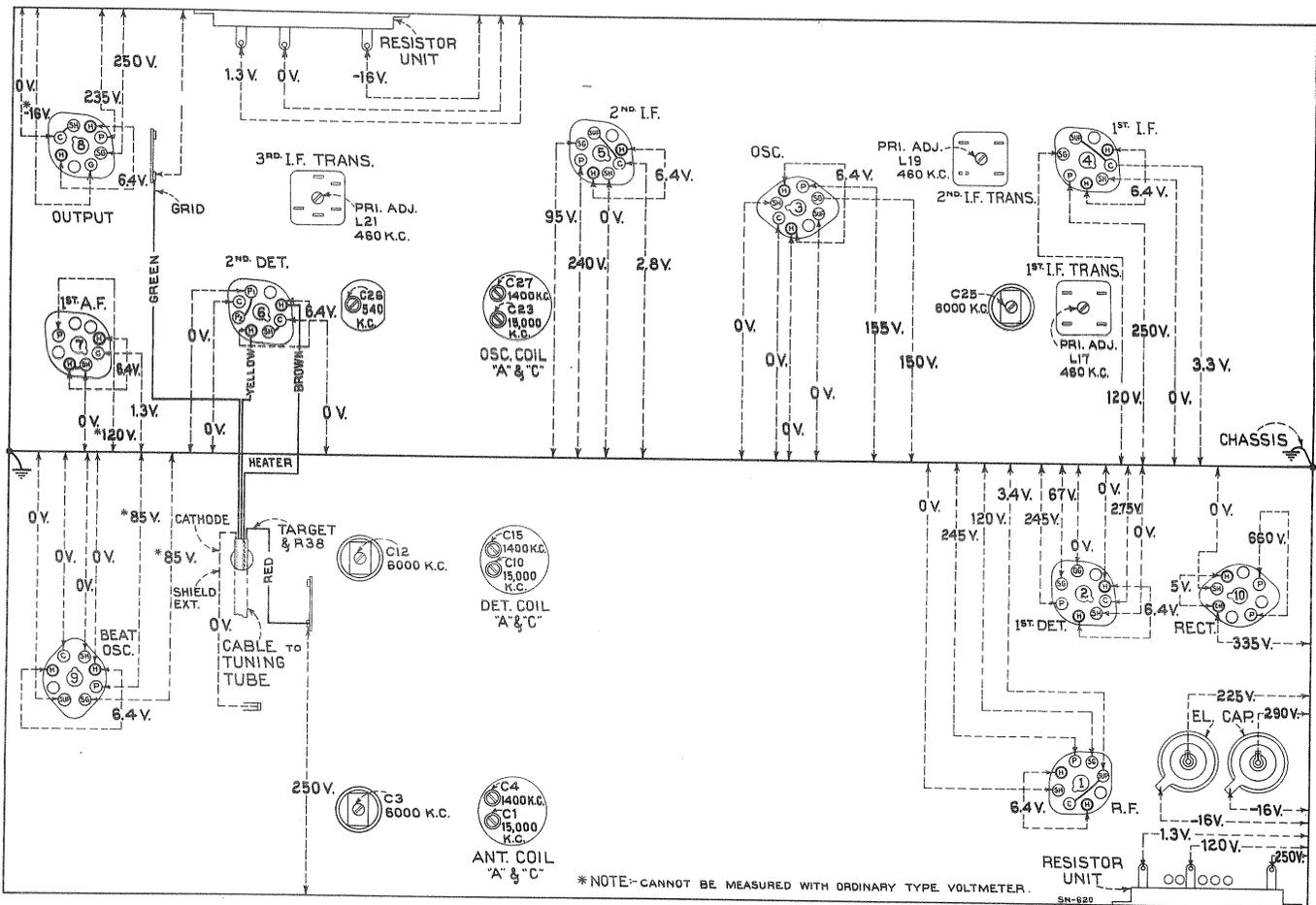
All voltages are measured with the Sensitivity Control at "1" (fully clockwise), Beat-Oscillator "on," Crystal "off," AVC "on," Dial Pointer at 900 Band "A." Grid Cap voltages to ground are "zero," except for the two oscillators.
