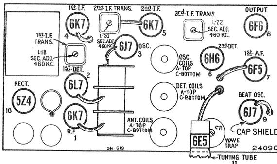
Figure 10—Radiotron and Coil Locations.
