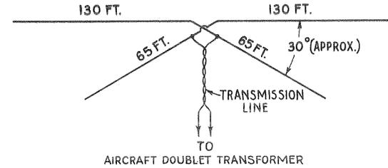
(c) Double Doublet Antenna for 160 and 80 Meter Bands
