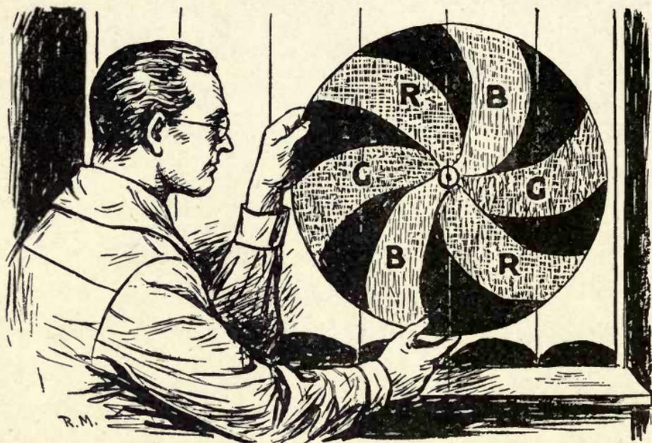
A DISK MADE UP OF FILTERS OF THREE DIFFERENT COLORS IS PLACED IN THE RECEIVER SET.
