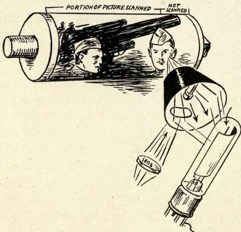
THIS IS ONE WAY OF SCANNING A PICTURE. THE LIGHT REFLECTED FROM EACH SPOT OF THE PICTURE SHINES UPON THE PHOTO-ELECTRIC CELL ON THE RIGHT.
