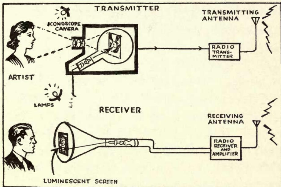
scope, the tube has an electron gun down in its narrow neck. The top of the tube is flat. It is made of a material that acts just the opposite from photo-electric material. Instead of producing electricity when light falls upon it, this material
