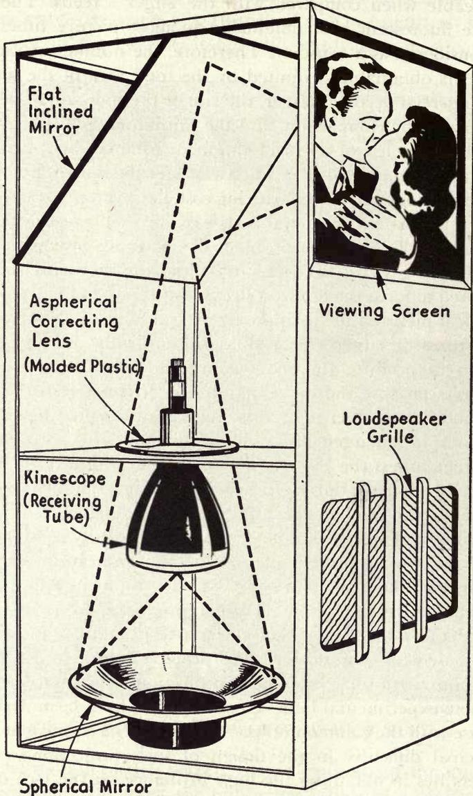
LARGE-SCREEN TELEVISION FOR THE HOME, DEVELOPED BY THE RCA LABORATORIES. Broken lines indicate the path of light beams from a single picture element on the face of the cathode-ray receiving tube to a corresponding point on the screen. A plastic lens is used to bring these light beams to a sharp focus on the screen
