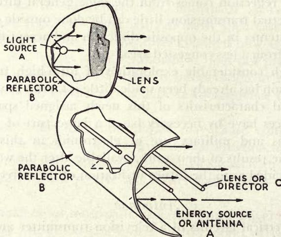
FIG. 1. PARABOLIC REFLECTORS
