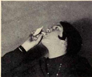
*The card can't be blown off by blowing through the spool (if the corners of your mouth don't leak)*
