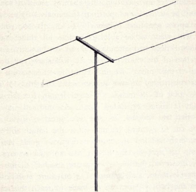
DIPOLE RECEIVING ANTENNA WITH REFLECTOR
