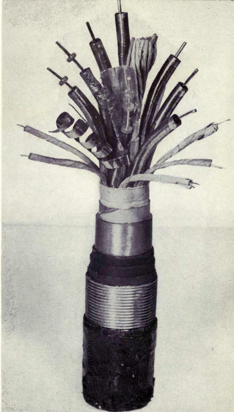
Typical coaxial cable showing the eight coaxial conductors (the large cylindrical tubes), and the secondary conductors which are used to carry control signals and power supply to the repeater or booster stations, located every 5 to 7 miles.
