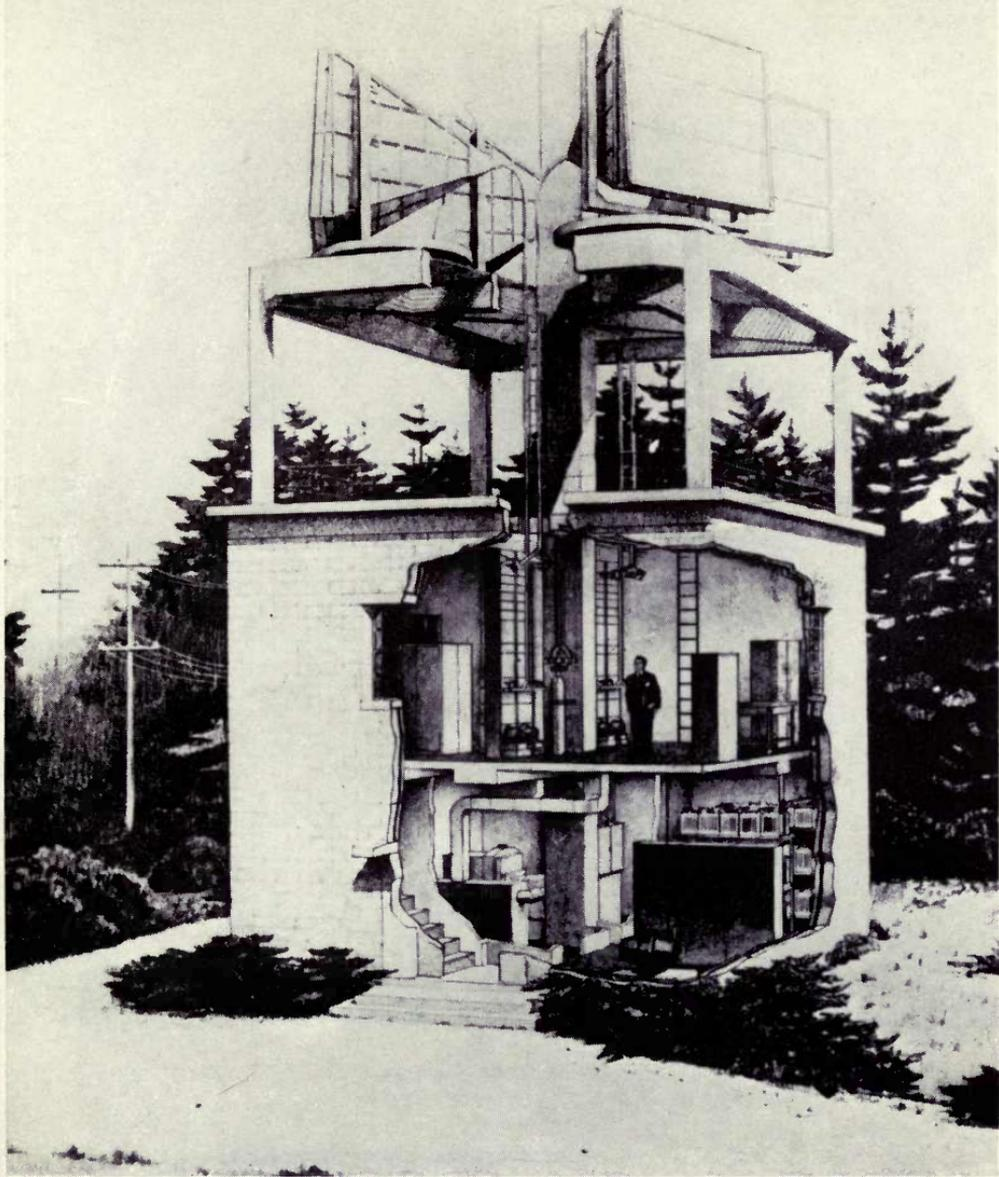
Cut-away view of one of seven radio relay stations on the Bell System radio relay route between New York and Boston, showing the arrangement of equipment in the building. Emergency power equipment and storage batteries are on the first floor, radio equipment on the second floor, and the microwave antennas which feature special electromagnetic lenses that receive and beam the communications signal, are on the roof.
