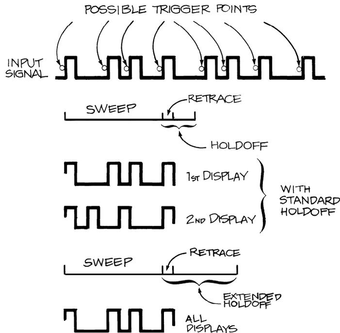
**Figure 12.** THE VARIABLE HOLDOFF CONTROL lets you make the scope ignore some potential trigger points. In the example, all the possible trigger points in the input signal would result in an unstable display. Changing the holdoff time to make sure that the trigger point appears on the same pulse in each repetition of the input signal is the only way to ensure a stable waveform.
