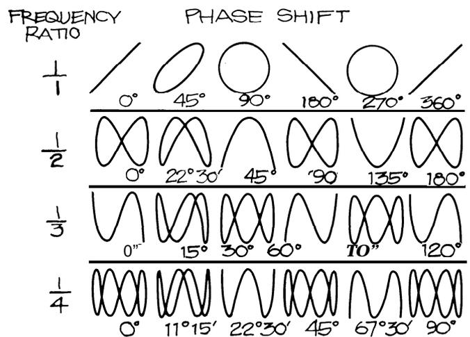
**Figure 26.** FREQUENCY MEASUREMENTS WITH LISSAJOUS PATTERNS require a known sine wave on one channel. If there is no phase shift, the ratio between the known and unknown signals will correspond to the ratio of horizontal and vertical lobes of the pattern. When the frequencies are the same, only the shifts in phase will affect the pattern. In the drawings above, both phase and frequency differences are shown.
