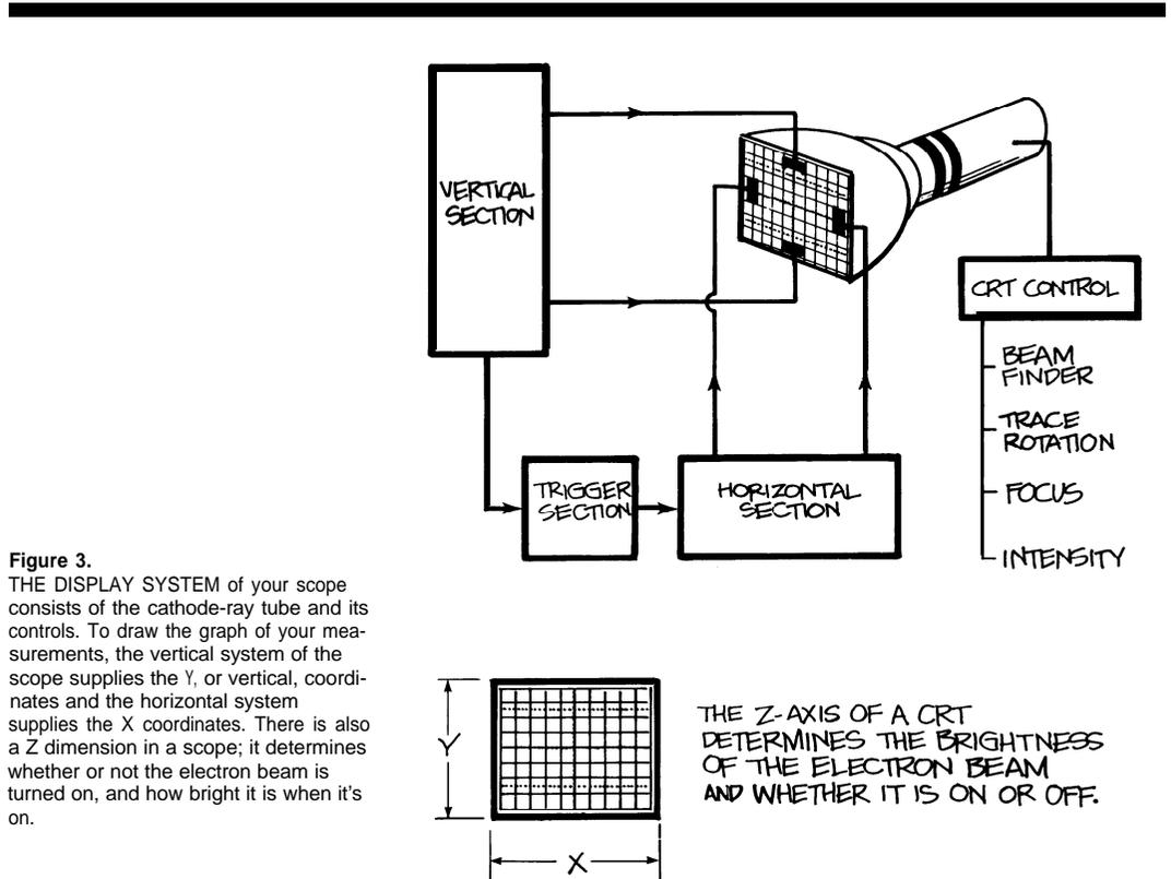
**Figure 3.** THE DISPLAY SYSTEM of your scope consists of the cathode-ray tube and its controls. To draw the graph of your measurements, the vertical system of the scope supplies the Y, or vertical, coordinates and the horizontal system supplies the X coordinates. There is also a Z dimension in a scope; it determines whether or not the electron beam is turned on, and how bright it is when it's on.
