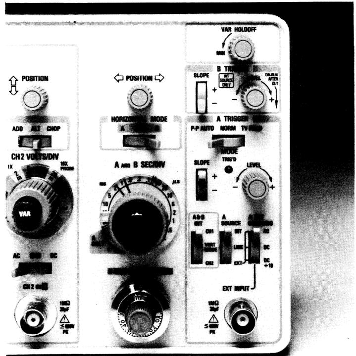
**Figure 30.** THE DELAYED SWEEP CONTROLS of the dual time base 2215 are shown on the photograph above. They include: HORIZONTAL MODE (under the horizontal POSITION control); B TRIGGER SLOPE and LEVEL; ALT SWP SEP (alternate sweep separation, between the two vertical POSITION controls — not shown), and a concentric A and B SEC/DIV control. The B DELAY TIME POSITION dial is at the bottom of the column of horizontal system controls.
