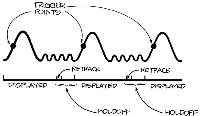
**Figure 11.** TRIGGER HOLDOFF TIME ensures valid triggering. In the drawing only the labeled points start the display because no trigger can be recognized during the sweep or the retrace and holdoff period. The retrace and holdoff times are necessary because the electron beam must be returned to the left side of the screen after the sweep, and because the sweep generator needs reset time. The CRT Z axis is blanked between sweeps and unblanked during sweeps.
