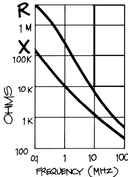
**Figure 15.** PROBE IMPEDANCE IS RELATED TO FREQUENCY as shown in the table above. The curves plot both resistance (R) and reactance (X) in ohms against frequency in megahertz. The plot shown is for the Tektronix P6120 probe on a 1-meter cable.
