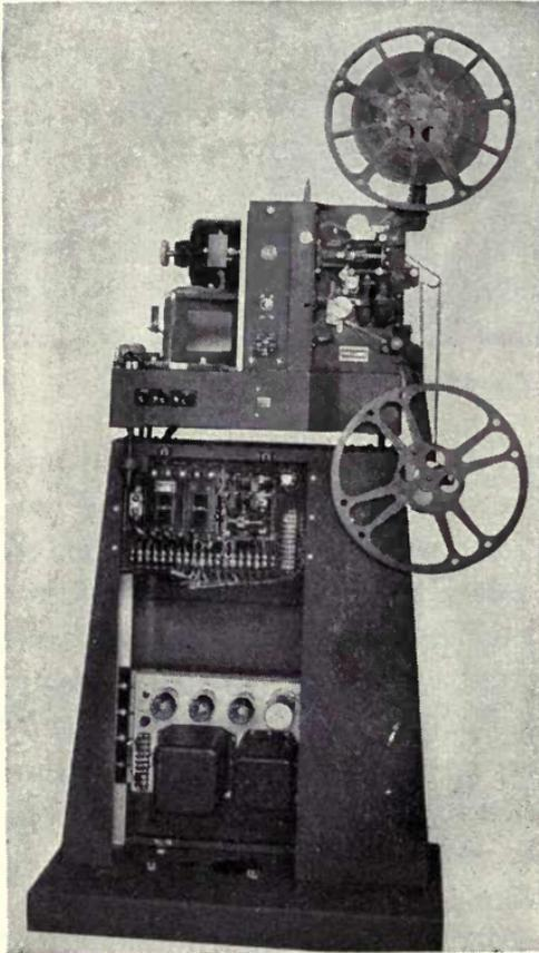
The RCA 16 mm Projector Figure 4-16 shows a "blown up" view of the equipment with the covers removed. The electronic equipment in the base is the power supply for the direct current to the three-phase motor field to ensure accurate synchronizing
