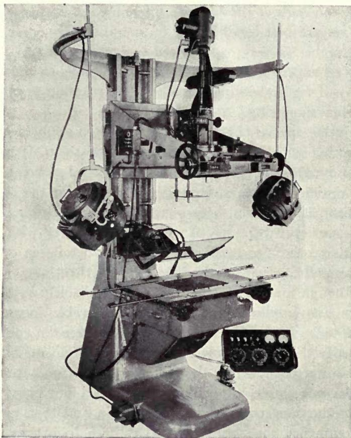
**Fig. 10-5. Acme Animation Stand.** Any lighting effect desired is possible with the table and lights shown. One to three films can be run through the camera at the same time. A foot control operates the camera leaving the operator's hands free. Zooms are possible of course, and the camera can be moved to follow any line or path desired. All types of effect can be made, including dissolves. Compressed air is used to move the camera and platen.
