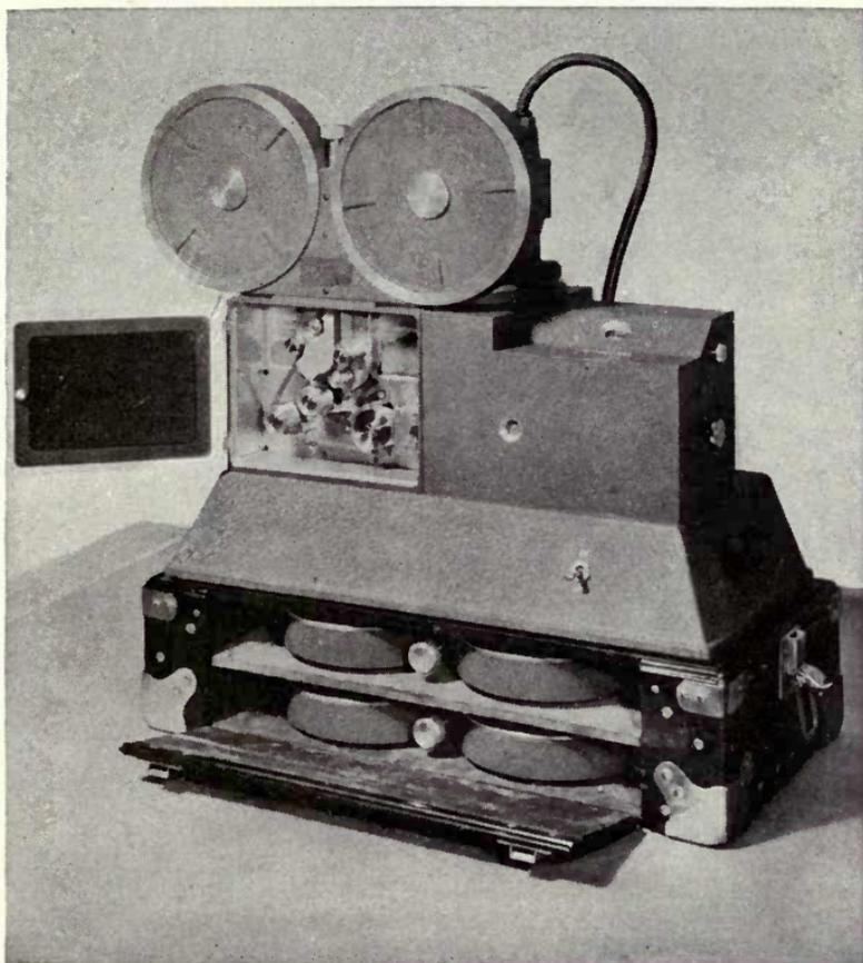
Fig. 3-15. Maurer sound recorder for 16 mm film showing spare magazines which are interchangeable with the camera magazines. The magazines shown hold film for eleven minutes (400 feet).
