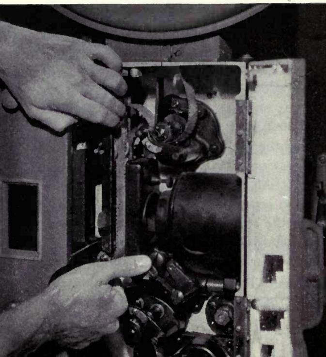
**Fig. 4-13A. Threading RCA 35 mm projector.**
