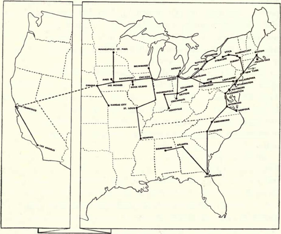
Fig. 19-1. The television cross-country lineup showing present and projected connections by coaxial cable and micro-wave relay link.
