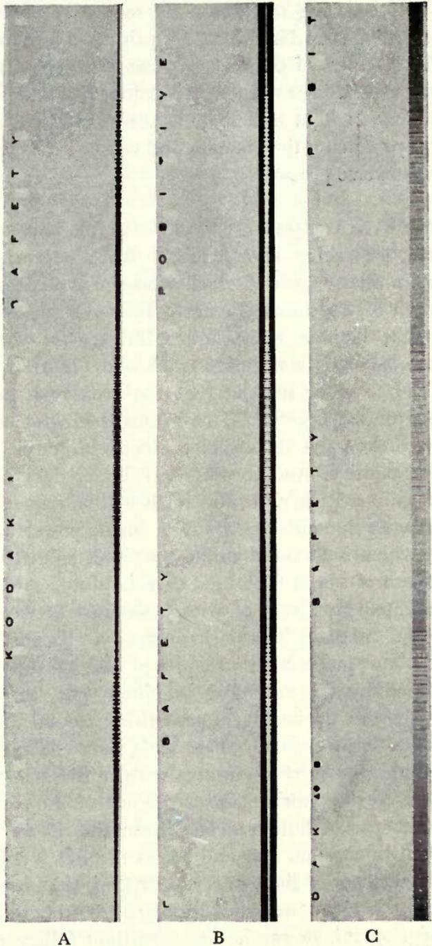
Fig. 3-13. Sound tracks of variable-area and variable-density recordings. Left (A) is variable-area negative, center (B) is variable-area positive, and right (C) is variable-density.
