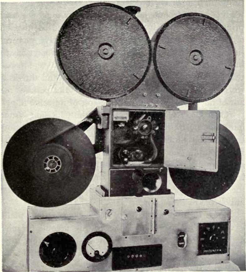
Fig. 10-2. Acme Contact Printer for 35 mm film. A 16 mm model is also available. The unexposed film is contained in the upper magazine. As the processed stock and the raw stock pass in front of the printing light the two emulsions are in contact. Notches in the processed film control the light intensity to correct for exposure variations. Up to forty feet of film a minute can be printed.
