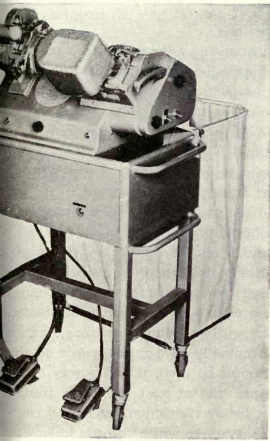
Fig. 9-4, A and B. Moviolas for sound editing and synchronizing 16 mm film.
