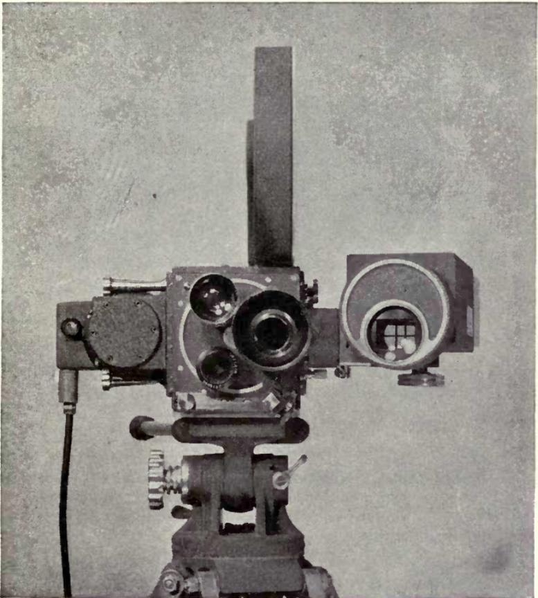
Fig. 3-9. The Maurer 16 mm camera for silent work as seen from the actor's position. Note the view finder on the right.
