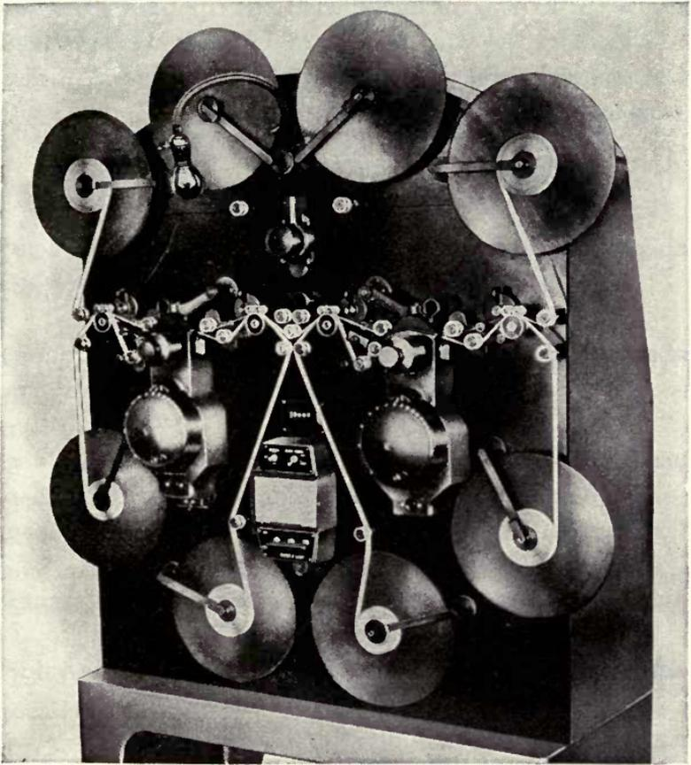
Fig. 1-3. Houston contact printer for 16 mm film.
