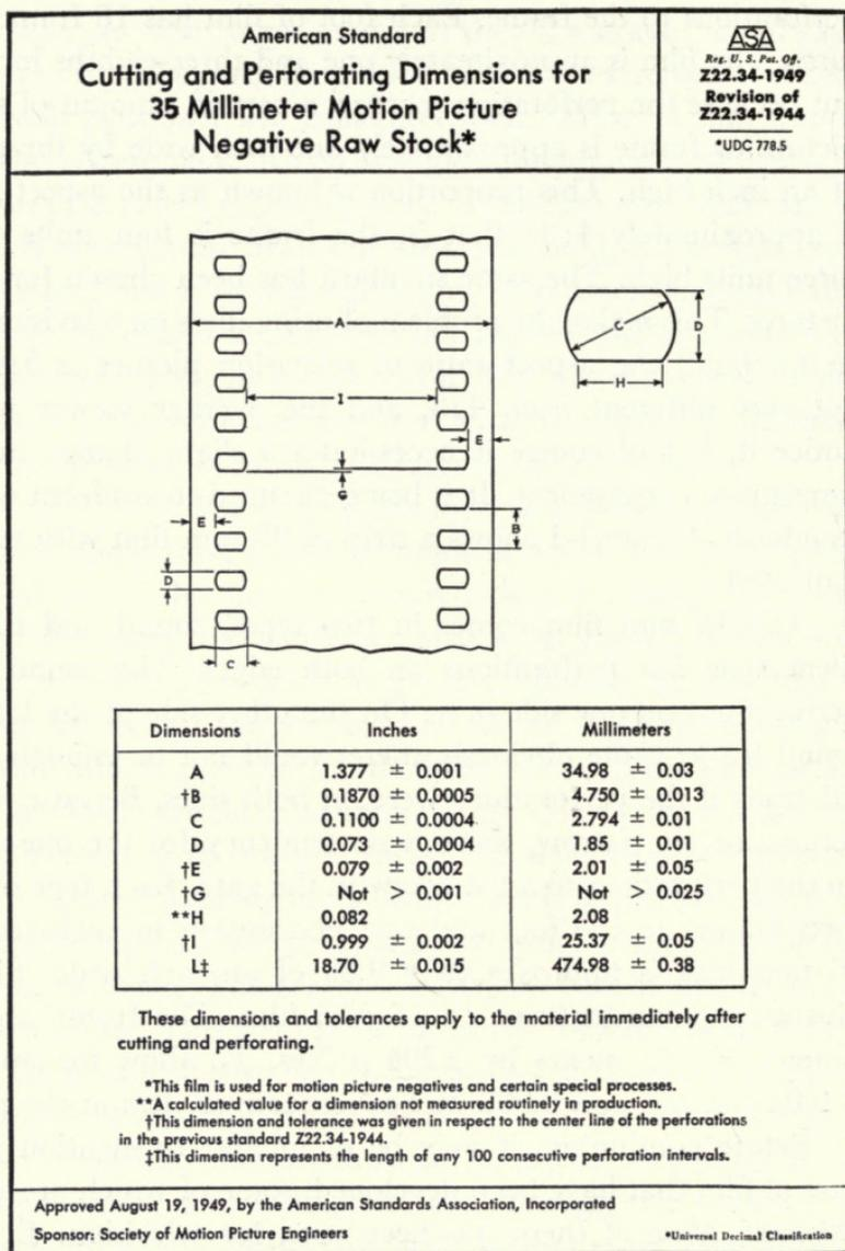
**Fig. 1-1. Dimensions and details of 35 mm film stock showing perforations and general appearance. Frame size (camera) 0.868 by 0.631 inches. Projector aperture is 0.825 by 0.600 inches.**
