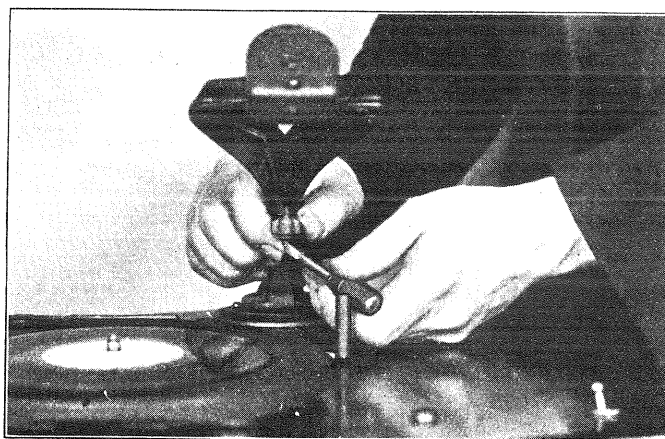
Figure 7—Adjusting Tone Arm Lowering Screw
