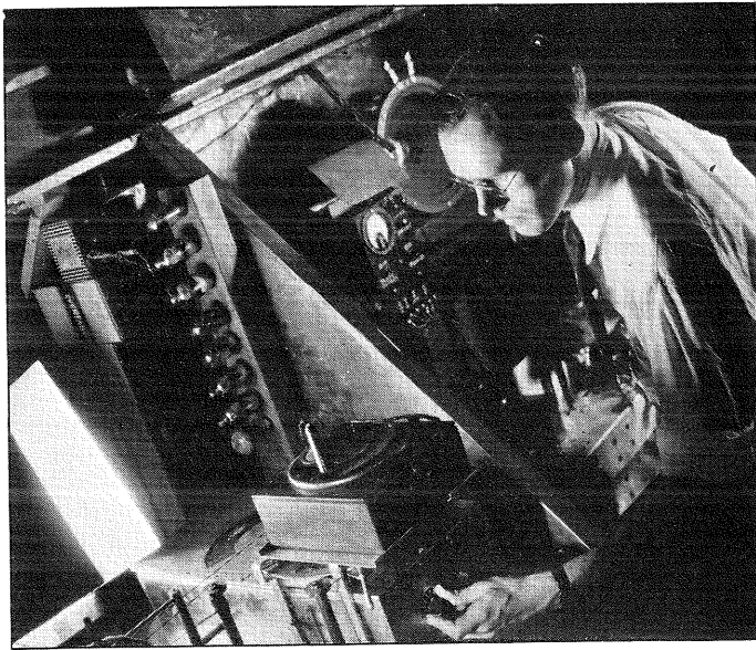
Drawing I. F. curves by means of specially developed equipment
