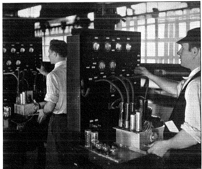
The continuity test—one of many tests along the production line
