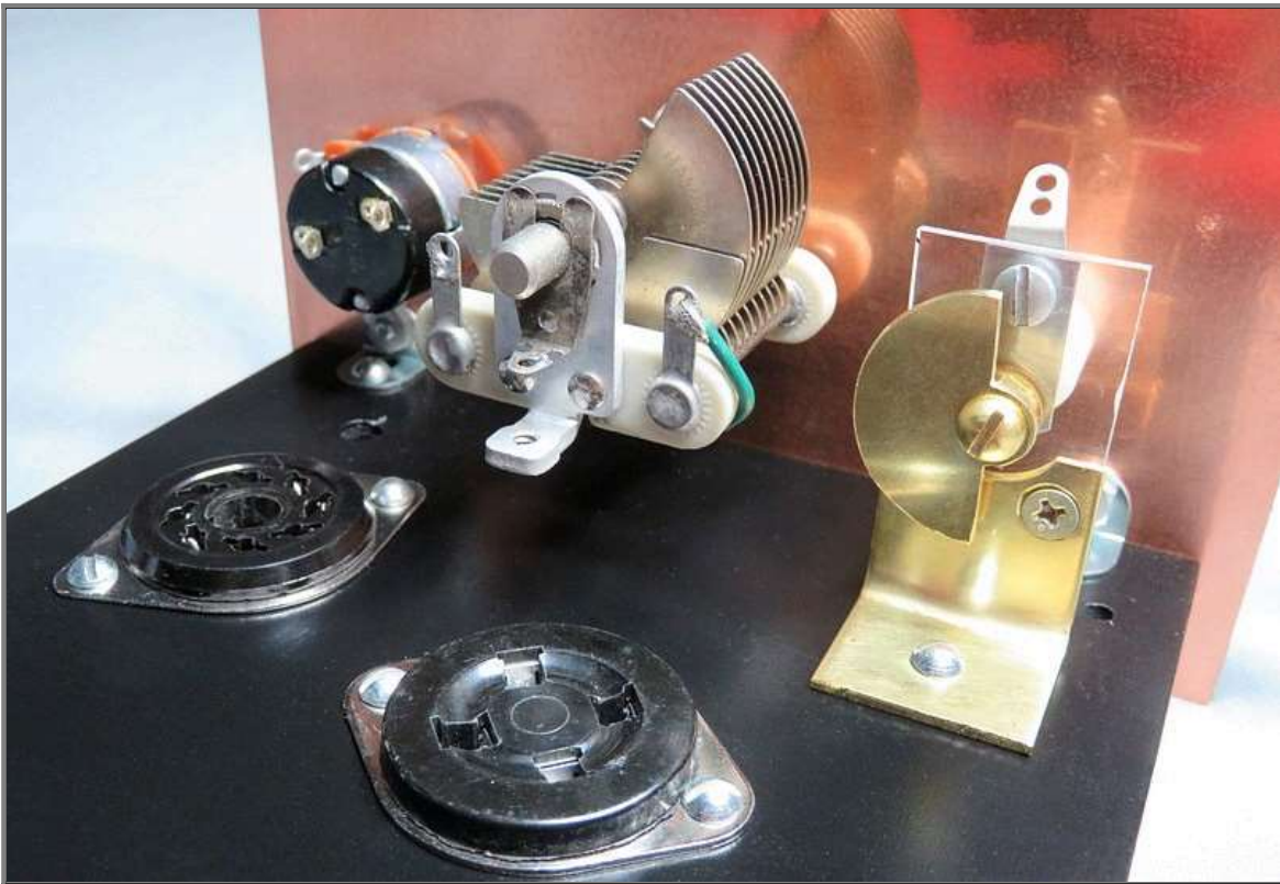
Parts mounted on the front panel and base. Because Sloan Freeman made me paranoid about the "conducting paint," the bottom of the antenna tune cap is covered with a piece of tape. The screw goes through an oversized hole and a mica washer prevents the nut from contacting the bottom of the base.
