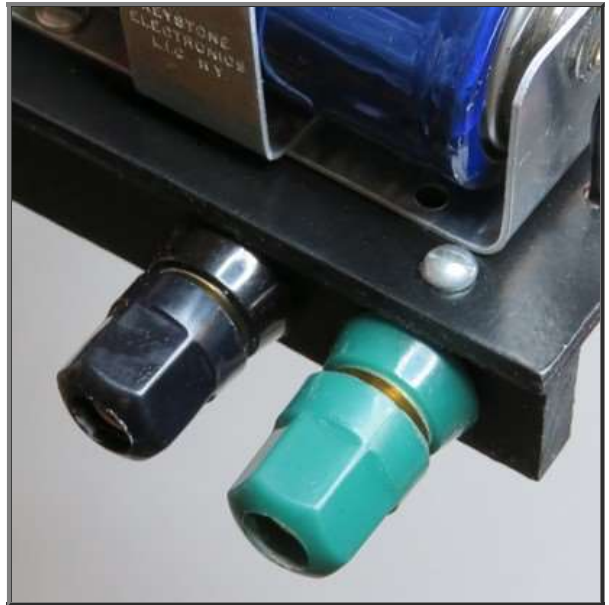
I also swapped my cool homemade binding posts with ones that don't conduct to the chassis.
