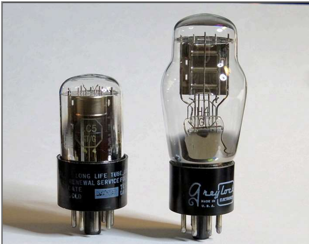
Before we test the radio, let's look at the two different vacuum tubes. MRL used a 1C5. Alfred Morgan used a 1H4. What are the differences?
