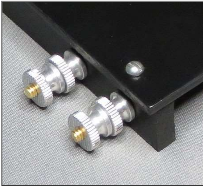
I also swapped my cool homemade binding posts with ones that don't conduct to the chassis.
