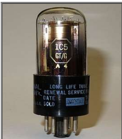
The 1C5 is a Pentode . Filament voltage is 1.4 volts @ .1 amp Pin 3 is the plate, pin 4 is the screen grid, pin 5 is the control grid.
