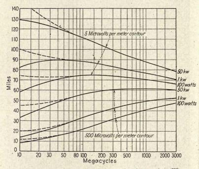
Fig. 115.—Signal range for high-frequency broadcast stations (IV).
