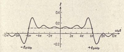
Fig. 36.—Response of the filter of Fig. 34 to the square pulse, with c=0.1 and  $\phi=0$ . The peak-to-peak amplitude is 0.5. The gain in signal to noise at the top frequency is 7.5 db, the loss at zero frequency 12.5 db.
