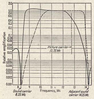
Fig. 28.—Picture amplifier characteristic. (R. D. Kell.)
