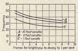
Fig. 59.—Same as Fig. 55, but frequency vs. number of frames required for brightness decay to one per cent. (A. V. Bedford.)
