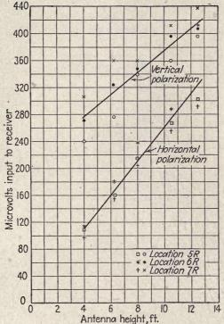
Fig. 104.—Field survey of signal strength, 69 Mc, comparing horizontal and vertical polarization. (W. L. Carlson.)
