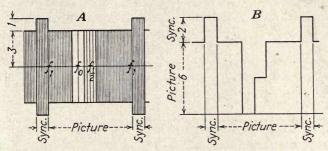
Fig. 70.—Transmitter-output waveforms, method 5. (R. D. Kell.)
