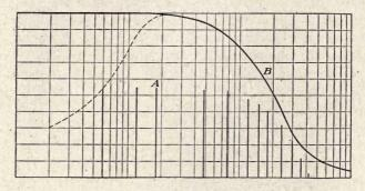
Fig. 86.—(A) Calculated wave analysis of the low-frequency type of pulse; (B) calculated response of low-frequency selector circuit. (Campbell and Lempert.)
