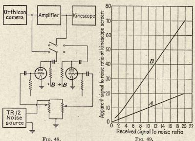
Fig. 48.—Test setup for determining television-brightness-transfer characteristics. (R. D. Kell.)
