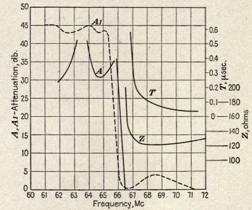
Fig. 21.—Time delay (T), attenuation (A, A'), and characteristic impedance (Z), of the Farnsworth vestigial sideband filter.  $(R. F. \ Wild.)$
