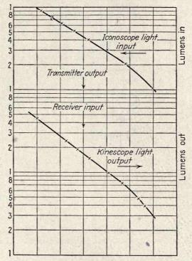
Fig. 47.—Combined transmitter and receiver transfer characteristics from input light to output light. (R. D. Kell.)
