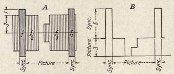
Fig. 69.—Transmitter-output waveforms, method 4. (R. D. Kell.)
