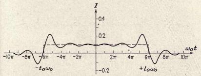
Fig. 41.—Response of the filter of Fig. 39 to the square pulse, for c=0.1 and  $\phi=0$ . The peak-to-peak amplitude is 0.34. The gain in signal to noise at the top frequency is 11 db, whereas the loss at zero frequency is 9 db.
