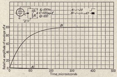
Fig. 91.—(A) Response of resonant circuit to square pulse; (B) response of resonant circuit to 500-kc square carrier pulse. (Campbell and Lempert.)
