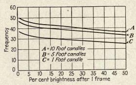
Fig. 60.—Same as Fig. 55, but frequency vs. percentage brightness after one frame. (A. V. Bedford.)
