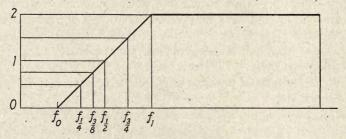
Fig. 65.—Idealized receiver-frequency characteristic. (R. D. Kell.)
