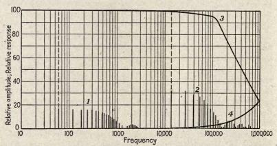
Fig. 90.—(1) Calculated harmonic analysis of the low-frequency wave, 700- $\mu$ see. duration, 60 c.p.s.; (2) calculated harmonic analysis of 8 per cent 13,230-c.p.s. horizontal synchronizing wave; (3) response curve, typical high-speed integration circuit; (4) response curve, 150- $\mu$ f 270-ohm differentiation circuit. (Campbell and Lempert.)
