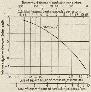
Fig. 62.—Sharpness of motion pictures at a viewing distance of 30 in. The frequency band is calculated on the basis of a 10- by  $7\frac{1}{2}$ -in. television picture, 30 frames per second, with 15 per cent horizontal and 7 per cent vertical blanking, under condition of equal vertical and horizontal resolutions. (M. W. Baldwin, Jr.)
