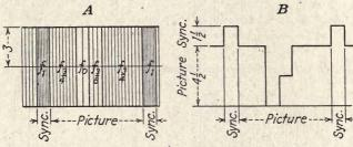
Fig. 67.—Transmitter-output waveforms, method 2. (R. D. Kell.)
