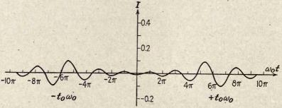
Fig. 43.—Response of the filter of Fig. 42 to the square pulse, for c=0 and  $\phi=0$ . Peak-to-peak amplitude 0.2. Gain in signal to noise at top frequency is 15.5 db; loss at zero frequency is infinite.
