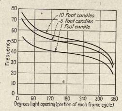
Fig. 55.—Degrees opening of sector disk vs. frequency for just-noticeable flicker.
