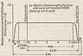
Fig. 1.—Idealized picture transmission amplitude characteristic.
