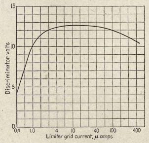
Fig. 16.—Limiter characteristic, taken at 2,859 kc. (center frequency 2,900 kc.), receiver X-563. (W. L. Dunn.)
