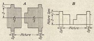
Fig. 66.—Transmitter-output waveforms, method 1. (R. D. Kell.)
