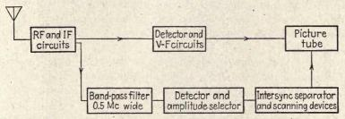
Fig. 75.—Receiver arrangement for the a-m and f-m interspersed signal.  $(A.\ V.\ Loughren.)$
