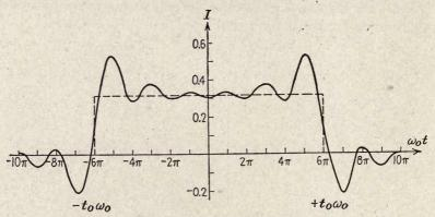
Fig. 37.—Response of the filter of Fig. 34 to the square pulse, for c=0.5 and  $\phi=0$ . The peak-to-peak amplitude is 0.735. The signal to noise gain at the top frequency is 4 db, whereas the loss at zero frequency is 6 db.
