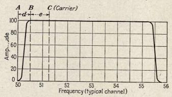
Fig. 18.—Amplitude characteristic of the picture transmitter, for receiverattenuation (RA) type transmission. (R. Serrell.)
