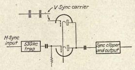
Fig. 81.—Circuit for removal of the 530-kc component in horizontal pulse. (Campbell and Lempert.)
