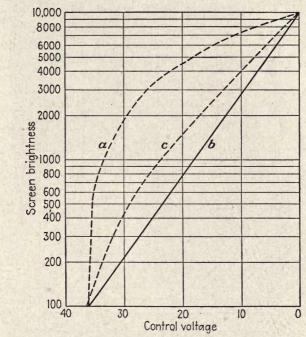
Fig. 45.—Comparison of receiver brightness-transfer characteristics: (a) linear system; (b) logarithmic system; (c) type 1803 kinescope. (R. D. Kell.)
