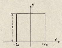
Fig. 30.—The square pulse applied to the input of the various filters. The pulse has unity amplitude and a duration of  $2t_o$ .
