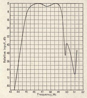
Fig. 12.—Actual response curve of vision channel from antenna to diode, receiver X-567 (No. 2), 44- to 50-Mc channel. (W. L. Dunn.)
