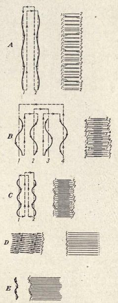
Fig. 53.—Effects of 120-c.p.s. ripple voltage on scanning-line positions, taken from Kell, Bedford, and Trainer. (A. V. Bedford.)
