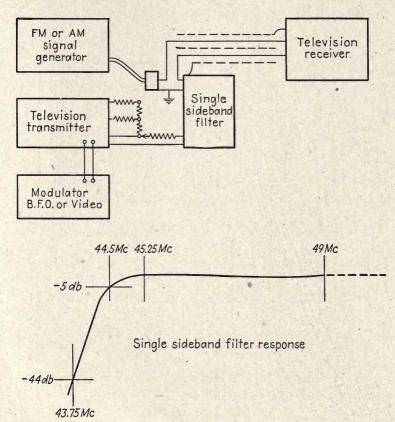
Fig. 17.—Block diagram of setup used in testing the use of f-m sound signals.
