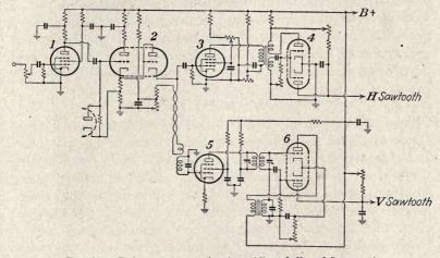
Fig. 87.—Pulse separator circuit. (Campbell and Lempert.)
