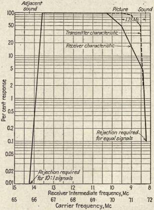
Fig. 6.—Picture and sound carriers "close spaced," i.e., 1.25-Mc separation.
