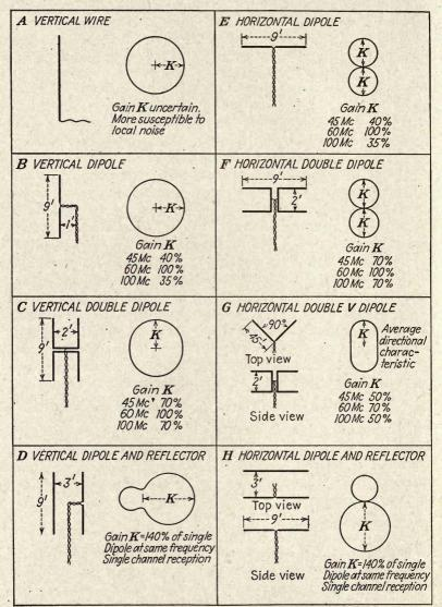
Fig. 100.—Various forms of outdoor television receiving antennas for vertical and horizontal polarization. (W. L. Carlson.)
